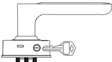
Method B: Use a mechanical key
