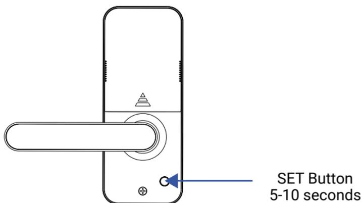
2. To configure a Siren as the responder, press and hold the SET button for 5-10 seconds until the LED quickly blinks green, then release the button.
