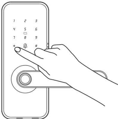
Method A: Press the "\*" button after unlock the door
