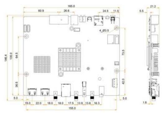
Tolerance: ±0.3 Unit: mm
