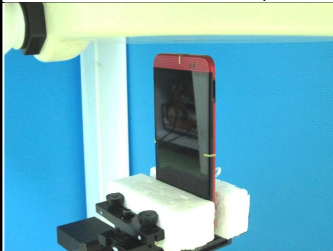
Top Side of EUT with 1.0 cm Gap
