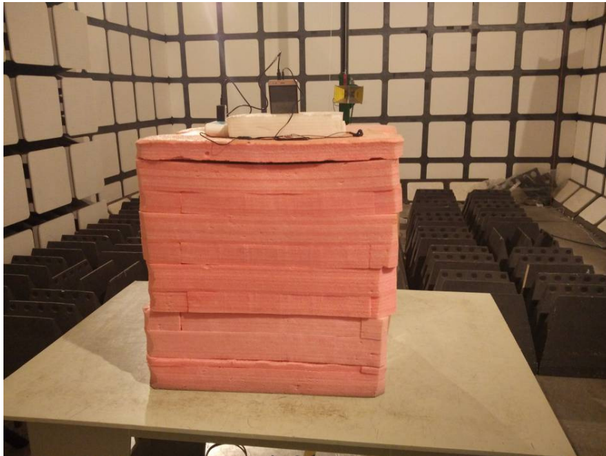
Radiated Emissions View (Above 1 GHz)
