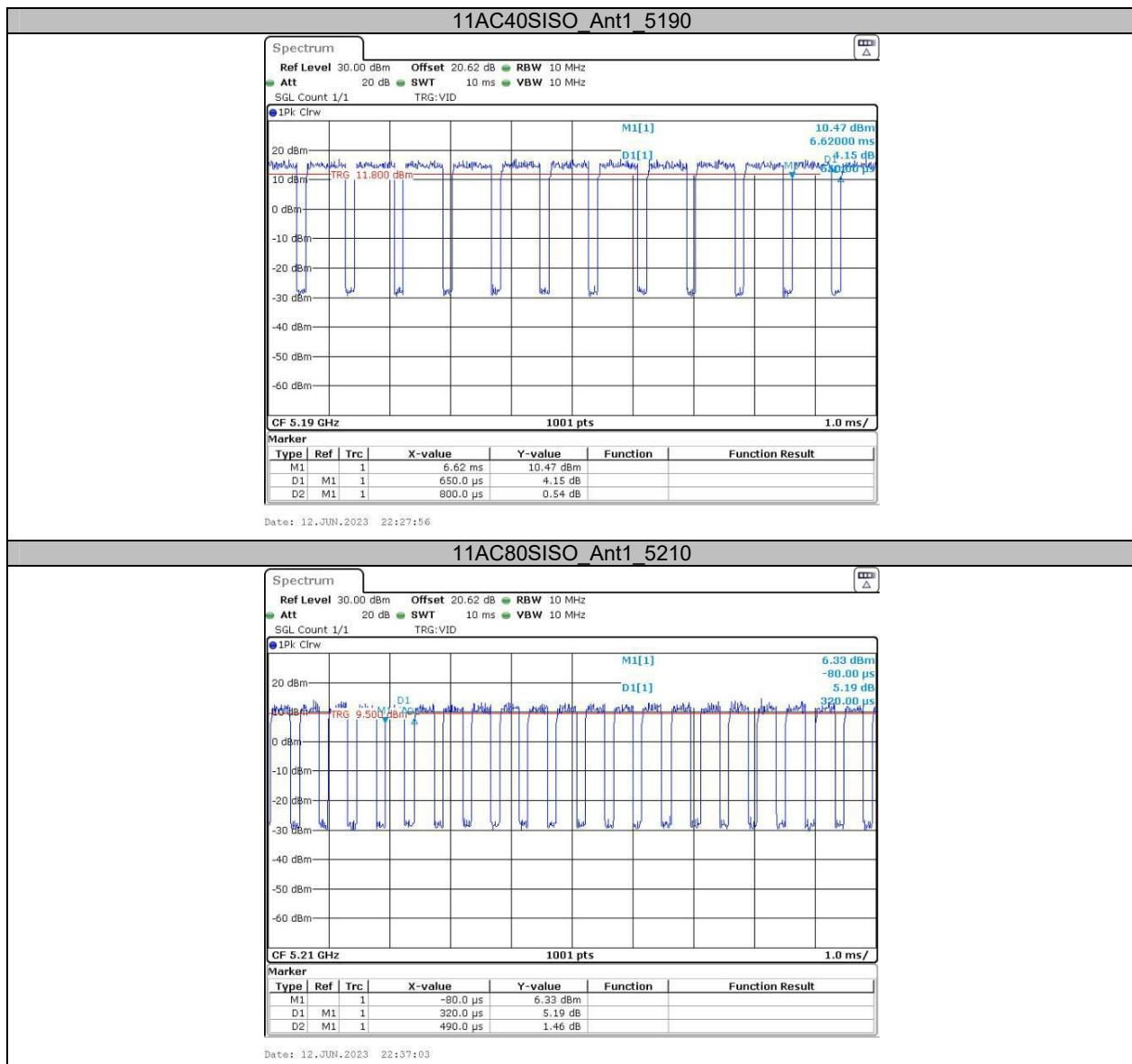
**Appendix C: Maximum conducted output power****Test Result**
