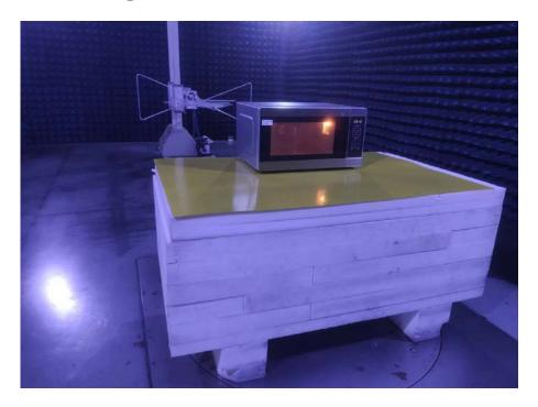
**Radiated Spurious Emissions Test View (Below 1GHz)**
