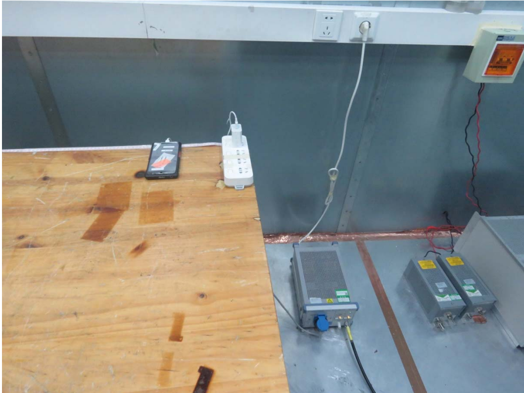
Picture 2 Conducted Emission Test Setup
