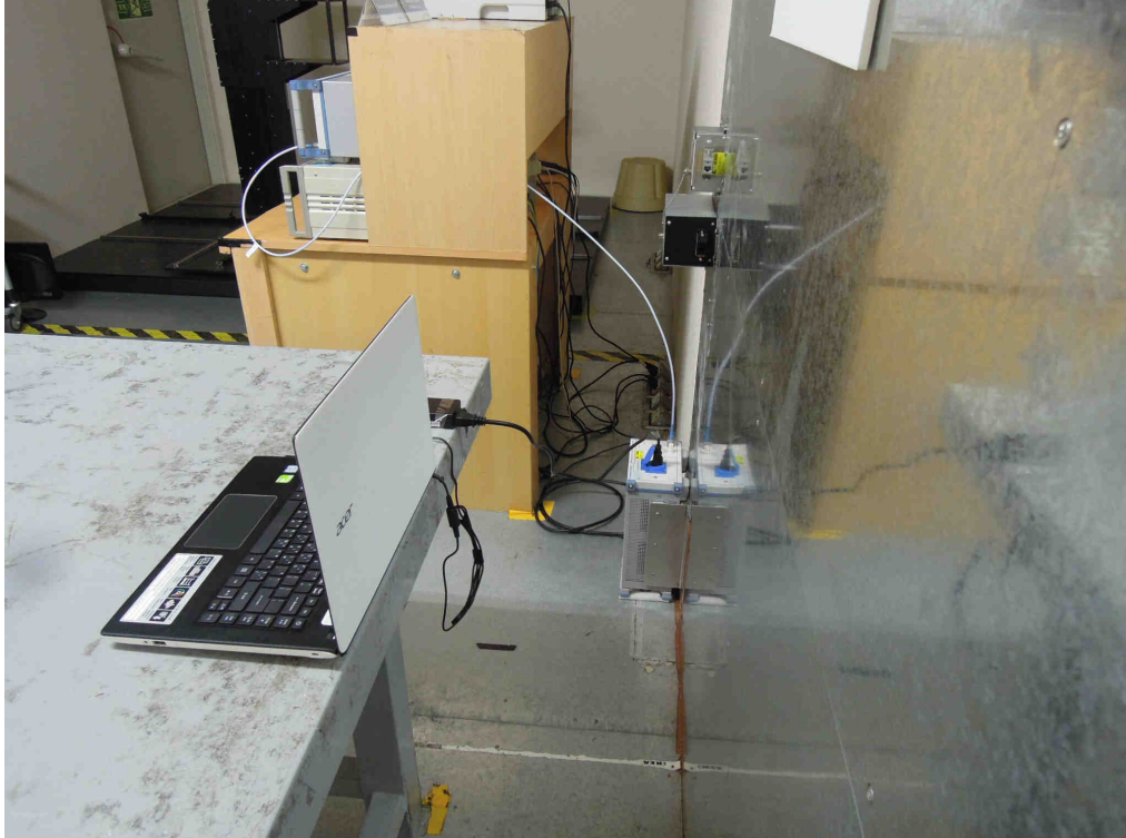
Photograph 4: Set-up for for Mains Conducted testing Back
