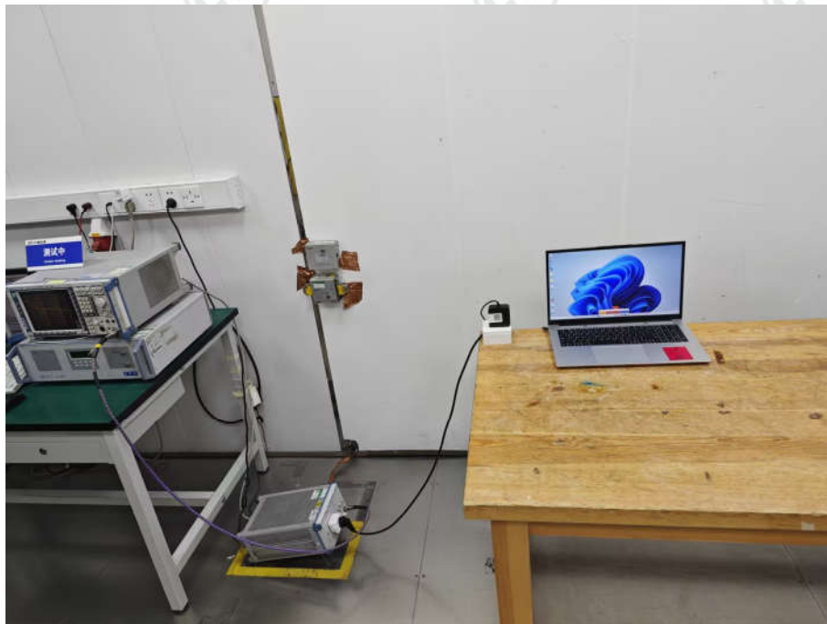
Conducted Emissions Test Setup
