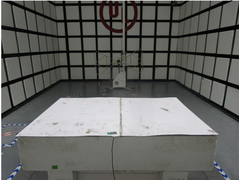
RADIATED RF MEASUREMENT SETUP (Below 30MHz)
