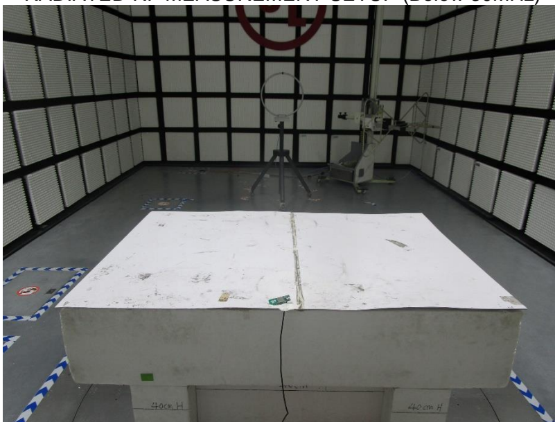
RADIATED RF MEASUREMENT SETUP (Below 30MHz)
