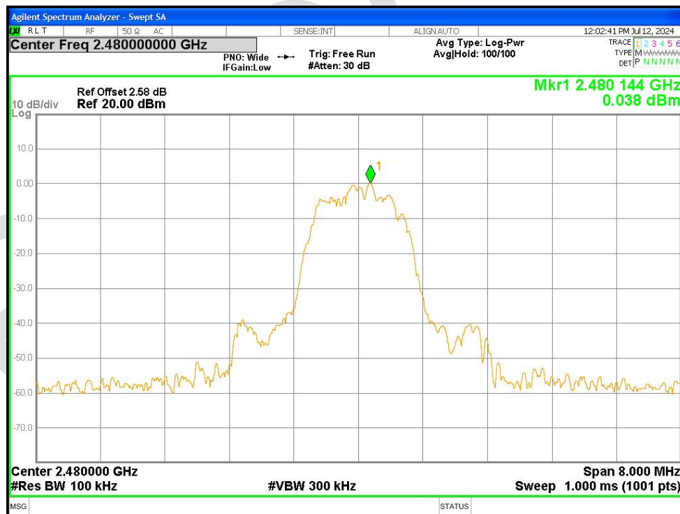
Band Edge NVNT 2-DH1 2480MHz Ant1 No-Hopping Emission
