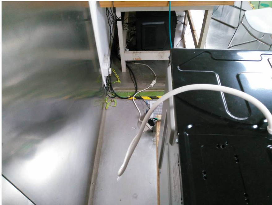
Conducted Emissions - Side View
