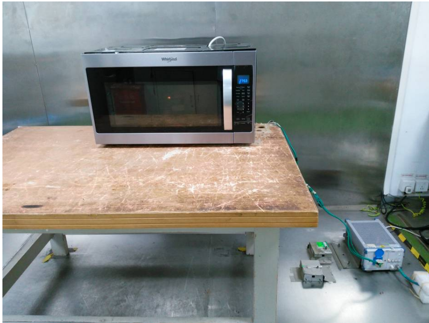
Conducted Emissions - Front View
