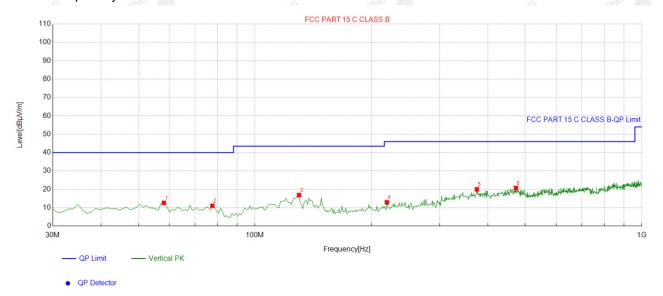
Suspected List Freq. Factor Reading Level Limit Margin Height Angle NO. Polarity [MHz] [dB]  $[dB\mu V/m]$ [dBµV/m]  $[dB\mu V/m]$ [dB] [cm] [°] 58.158158 -14.00 26.61 12.61 40.00 27.39 100 131 Vertical 77.577578 -18.02 29.03 11.01 40.00 28.99 100 326 Vertical 130.01001 -17.24 34.11 16.87 43.50 100 51 3 26.63 Vertical 219.33933 4 -14.60 27.56 12.96 46.00 33.04 100 142 Vertical 5 374.69469 -9.88 29.93 20.05 46.00 25.95 100 177 Vertical 472.76276 46.00 6 -8.35 29.11 20.76 25.24 100 358 Vertical
