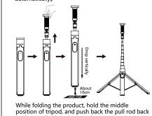
to the handle sleeve section by section.
