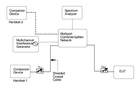
This test setup is used for all Monitoring and Time and Spectrum Access Procedure tests.
