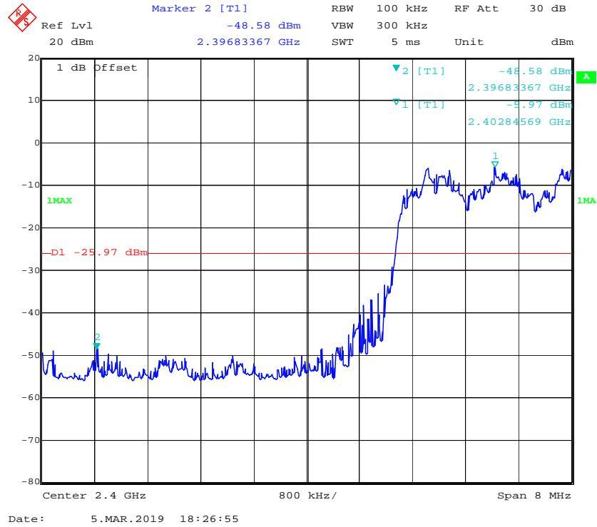
**Band Edge, Right Side**
