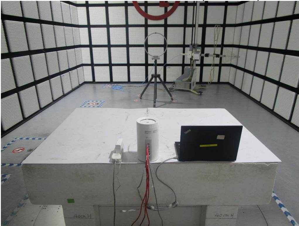
POWERLINE CONDUCTED EMISSIONS MEASUREMENT SETUP
