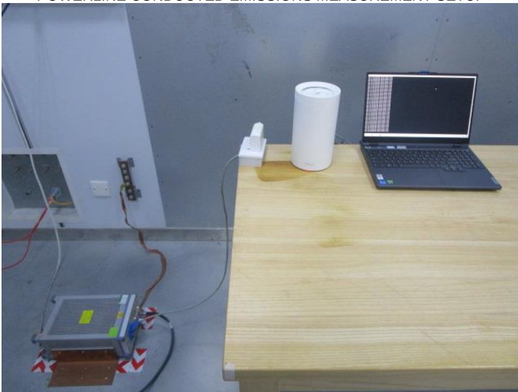
POWERLINE CONDUCTED EMISSIONS MEASUREMENT SETUP
