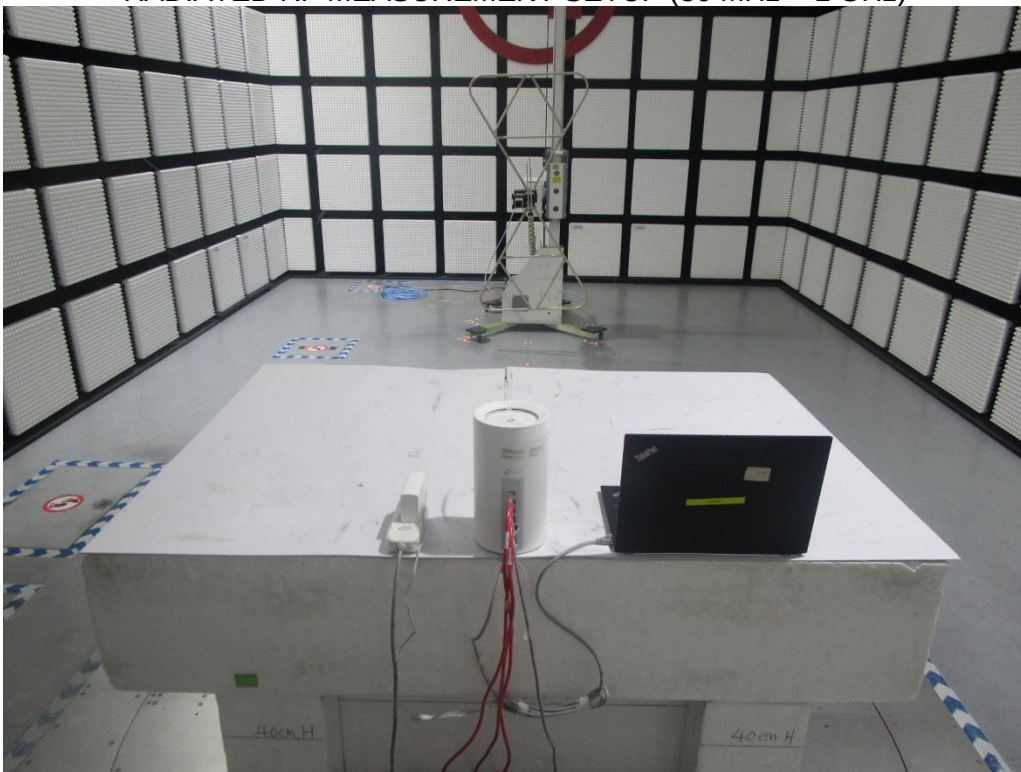
RADIATED RF MEASUREMENT SETUP (30 MHz ~ 1 GHz)
