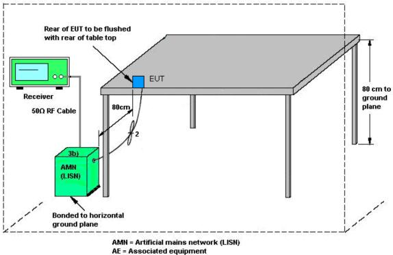
EUT = Equipment under test
