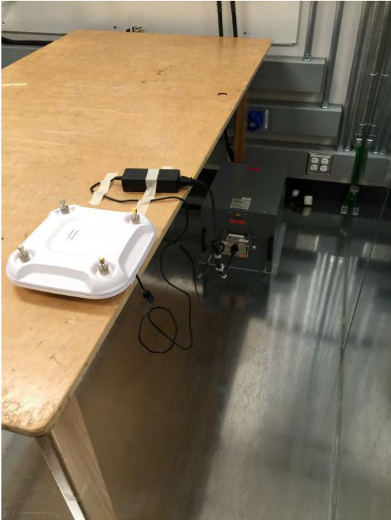
AIR-CAP3702P-B-K9 AC Conducted Emissions setup photo
