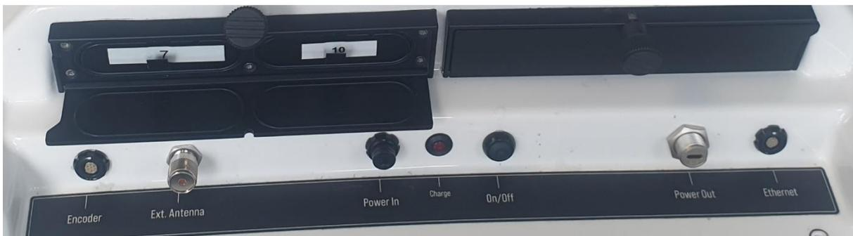
Photo 4: Connector panel with battery compartment one lid open. External Antenna connector for GPS antenna.
