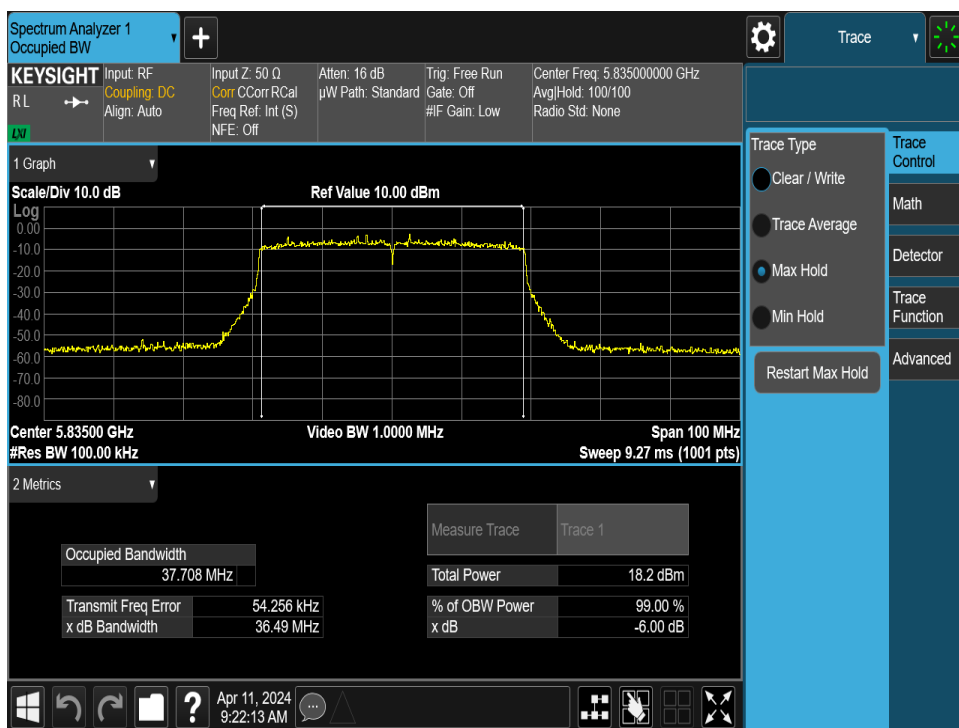
Plot 7-62. 6dB Bandwidth Plot MIMO ANT1 (40MHz BW 802.11ax/be (UNII Band 3/4) – Ch. 167)
