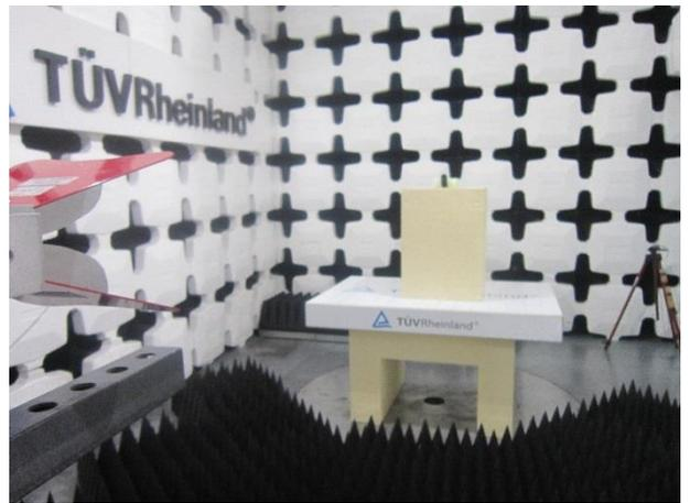
RADIATED TEST SETUP
