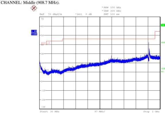
Note: The carrier was attenuated using a notch-filter. The peak shown in the plot is the carrier frequency.
