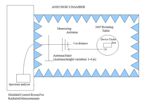
Radiated measurements setup f > 1 GHz
