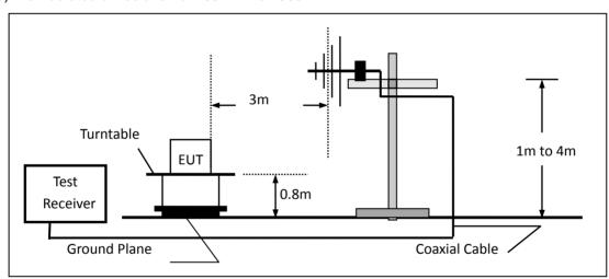
(c) For radiated emissions above 1000MHz
