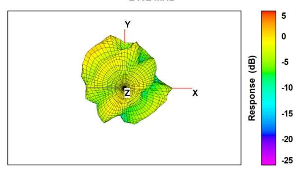
**OTA Test Results for Frequency 2440 MHz**
