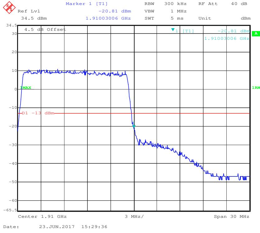
**QPSK (20.0 MHz, FULL RB) - Left Band Edge**
