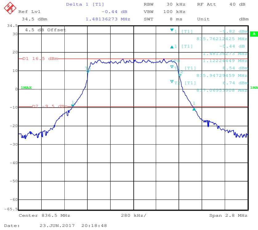
**16-QAM (1.4 MHz) - 99% Occupied Bandwidth &26 dB Bandwidth, Middle channel**
