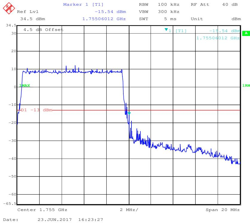
**QPSK (15.0 MHz, FULL RB) - Left Band Edge**
