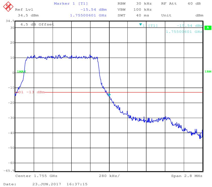
**16-QAM (1.4 MHz, FULL RB) - Left Band Edge**
