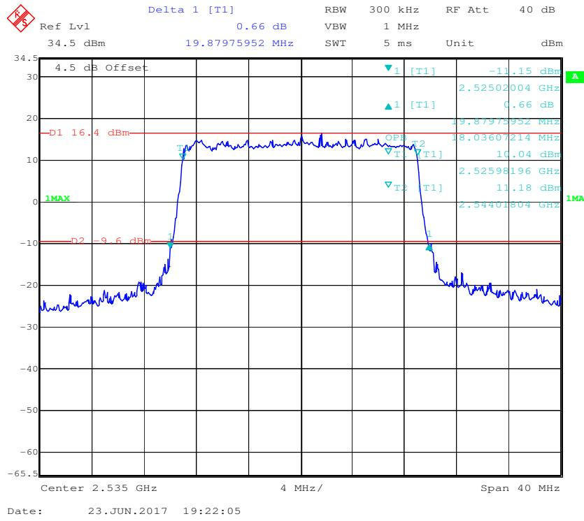
**16-QAM (20 MHz) - 99% Occupied Bandwidth &26 dB Bandwidth, Middle channel**
