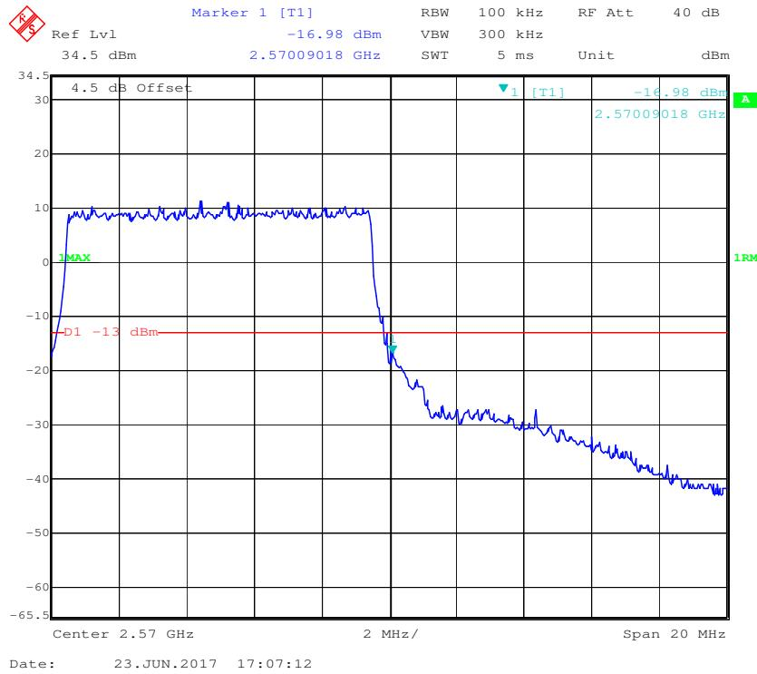
**QPSK (15 MHz, FULL RB) - Left Band Edge**
