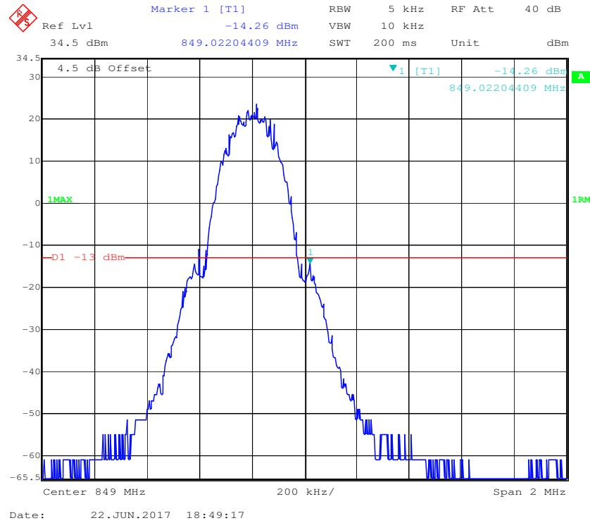
**Cellular Band, Left Band Edge for EDGE Mode**
