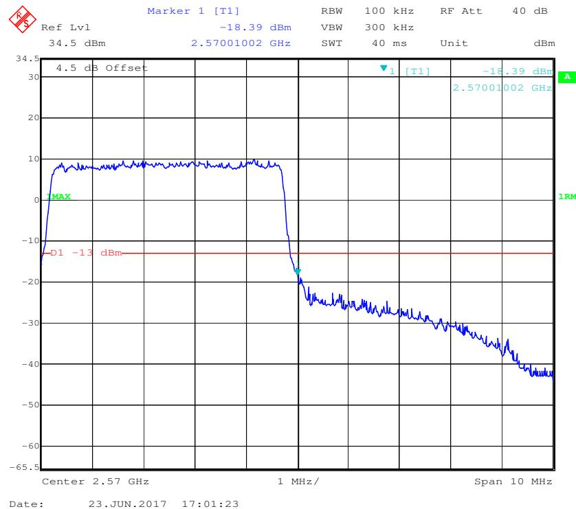
**16-QAM (5.0 MHz, FULL RB) - Left Band Edge**
