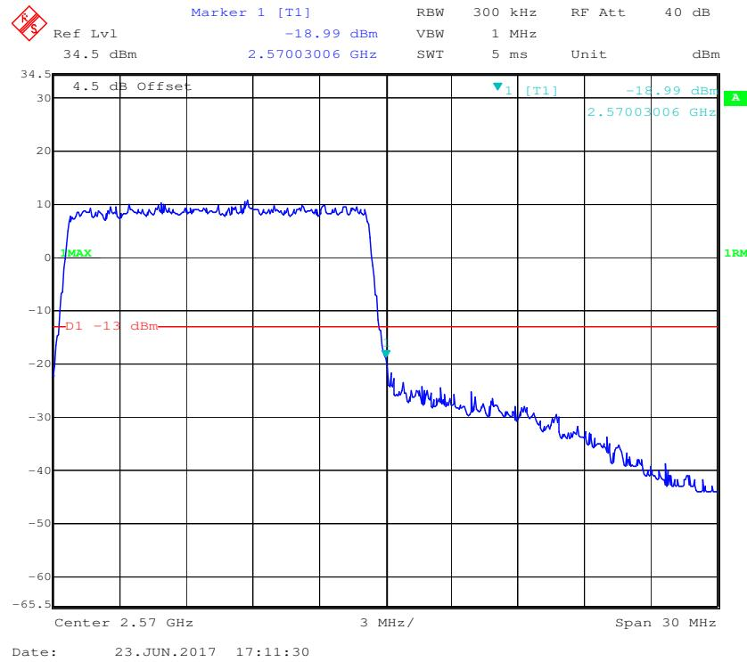
**QPSK (20 MHz, FULL RB) - Left Band Edge**
