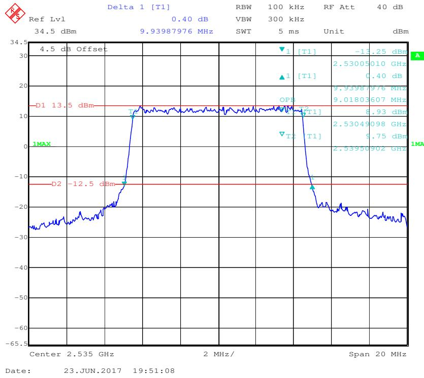
**16-QAM (10MHz) - 99% Occupied Bandwidth &26 dB Bandwidth, Middle channel**
