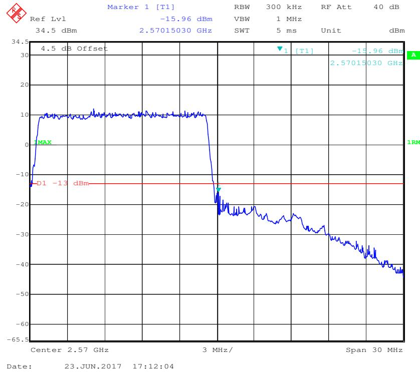
**16-QAM (15 MHz, FULL RB) - Left Band Edge**
