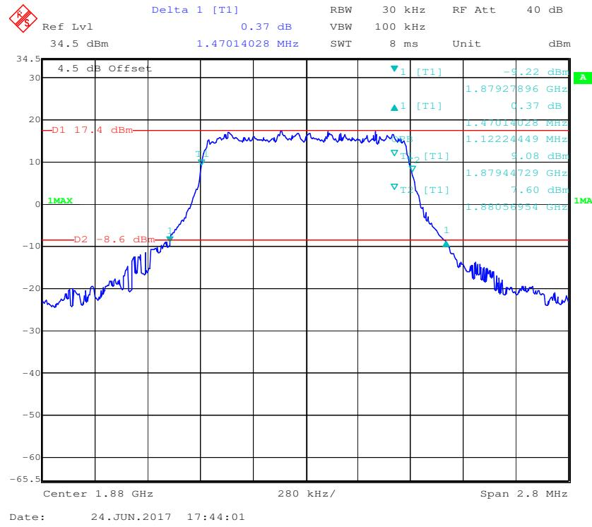
**16-QAM (1.4 MHz) - 99% Occupied Bandwidth &26 dB Bandwidth, Middle channel**
