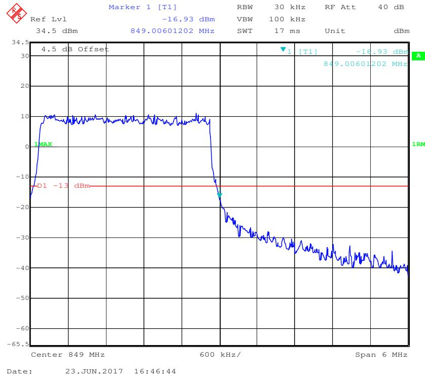
**16-QAM (3.0 MHz, FULL RB) - Left Band Edge**
