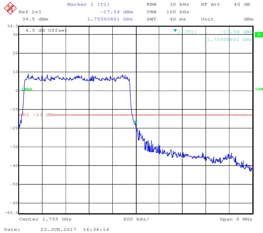
**16-QAM (3.0 MHz, FULL RB) - Left Band Edge**
