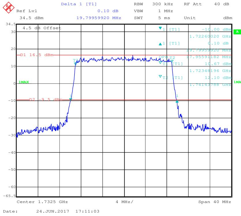
**16-QAM (20.0 MHz) - 99% Occupied Bandwidth &26 dB Bandwidth, Middle channel**
