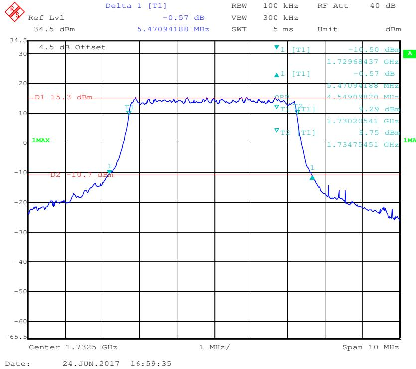
**QPSK (10.0 MHz) - 99% Occupied Bandwidth &26 dB Bandwidth, Middle channel**
