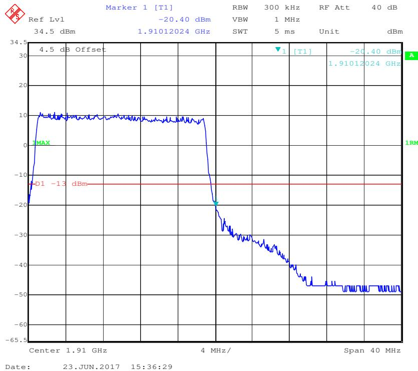
**16-QAM (20.0 MHz, FULL RB) - Left Band Edge**
