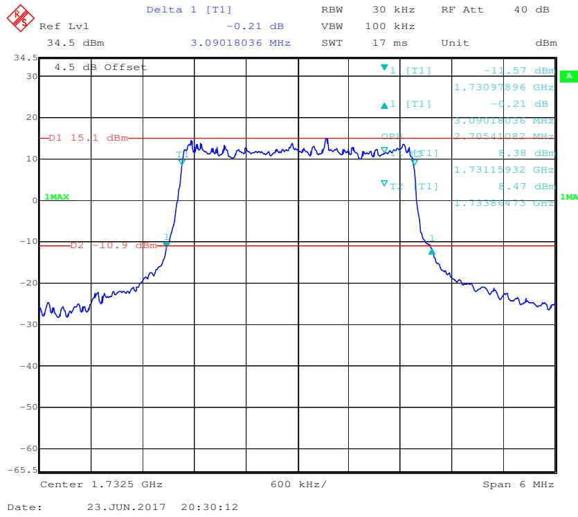
**16-QAM (3.0 MHz) - 99% Occupied Bandwidth &26 dB Bandwidth, Middle channel**
