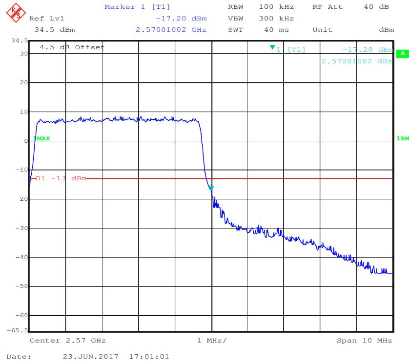
**QPSK (10.0 MHz, FULL RB) - Left Band Edge**
