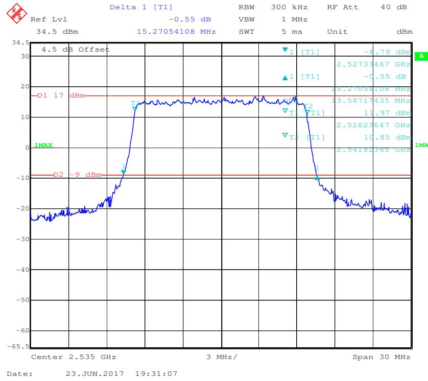
**16-QAM (15 MHz) - 99% Occupied Bandwidth &26 dB Bandwidth, Middle channel**
