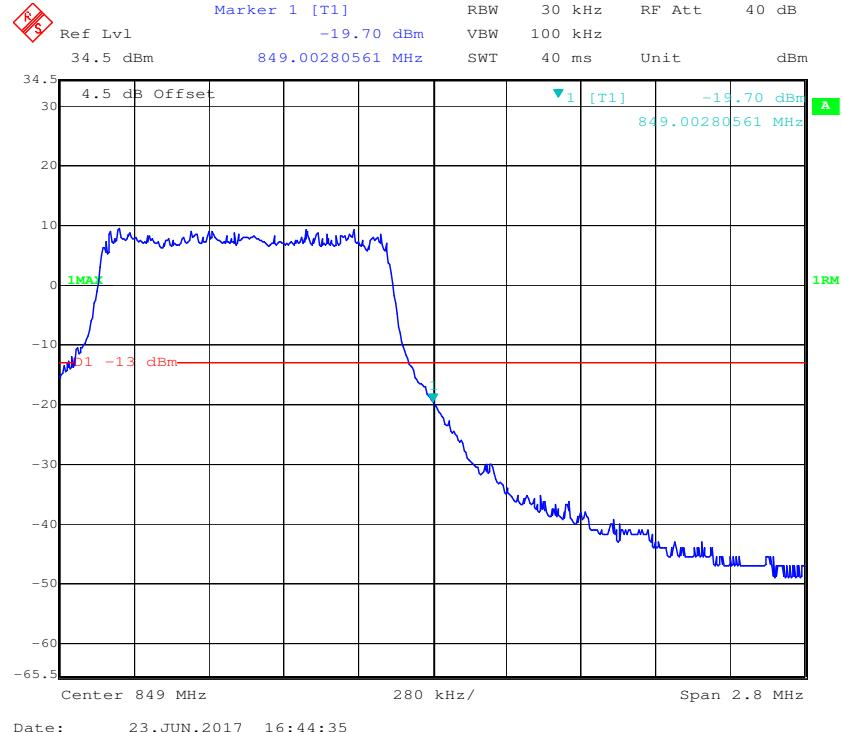
**QPSK (3.0 MHz, FULL RB) - Left Band Edge**
