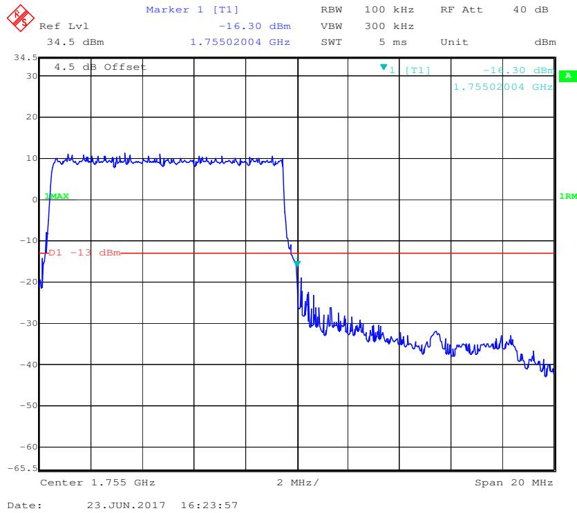
**16-QAM (10.0 MHz, FULL RB) - Left Band Edge**
