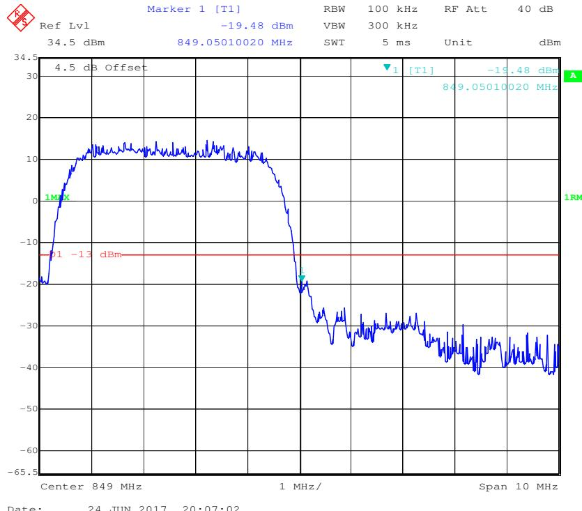
**Cellular Band, Left Band Edge for HSUPA (BPSK) Mode**
