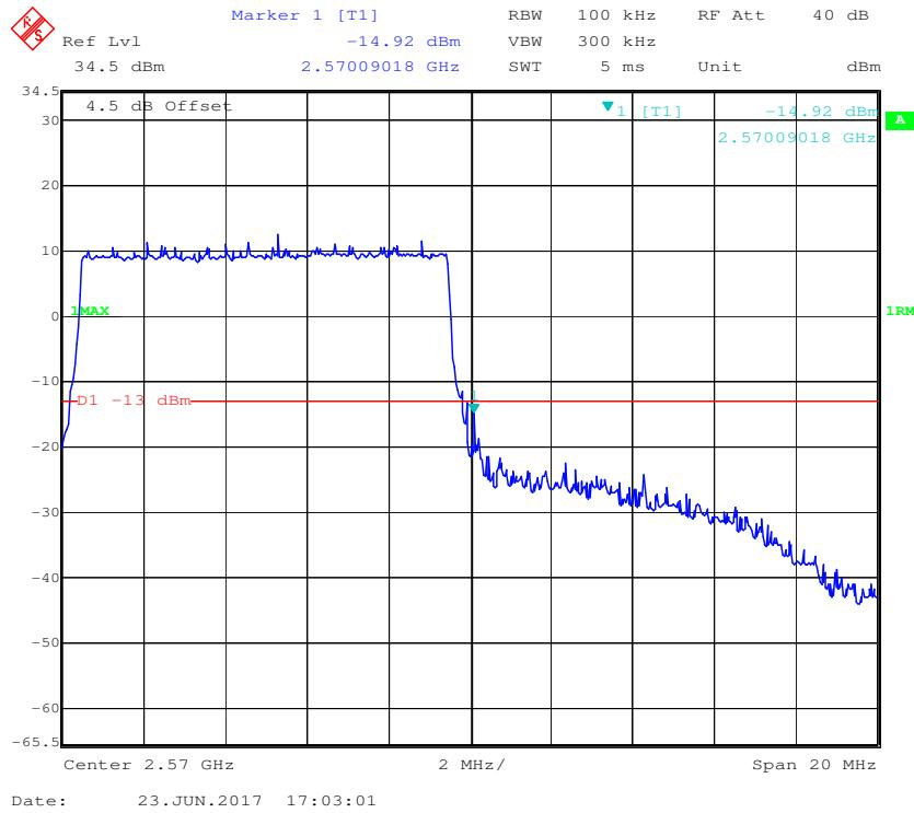
**16-QAM (10.0 MHz, FULL RB) - Left Band Edge**
