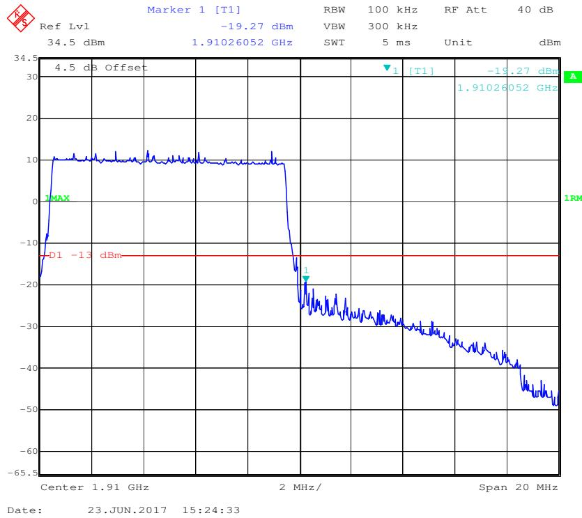
**16-QAM (10.0 MHz, FULL RB) - Left Band Edge**
