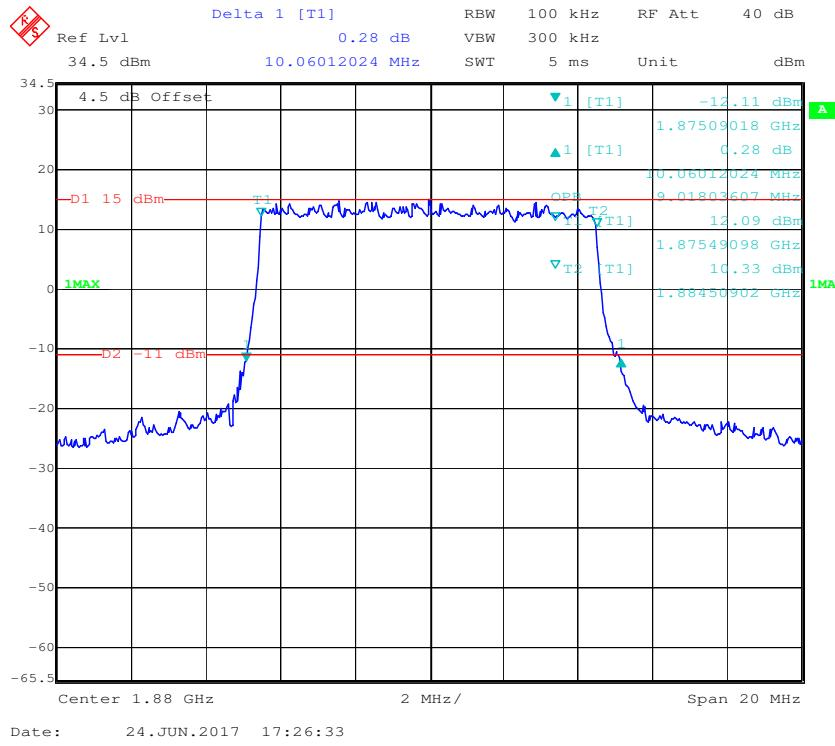
**16-QAM (10.0 MHz) - 99% Occupied Bandwidth &26 dB Bandwidth, Middle channel**
