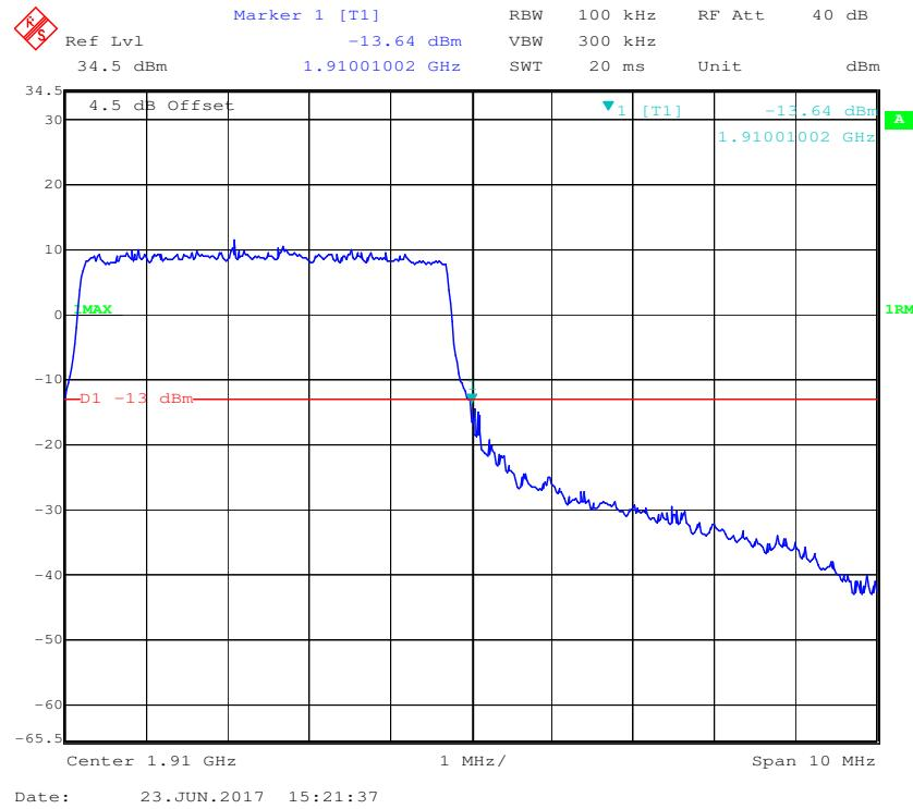
**QPSK (10.0 MHz, FULL RB) - Left Band Edge**
