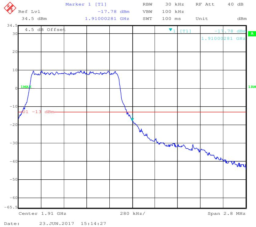
**QPSK (3.0 MHz, FULL RB) - Left Band Edge**
