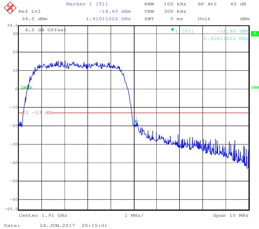
**LTE Band 2:****QPSK (1.4 MHz, FULL RB) - Left Band Edge**
