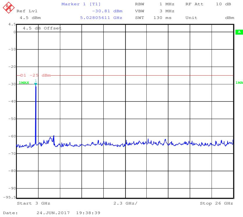
**FCC § 2.1053; § 22.917 (a);§ 24.238 (a); §27.53 (h)(m) SPURIOUS RADIATED EMISSIONS****Applicable Standard**
