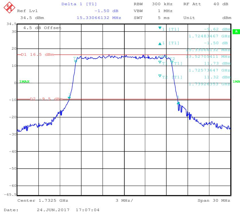
**16-QAM (15.0 MHz) - 99% Occupied Bandwidth &26 dB Bandwidth, Middle channel**
