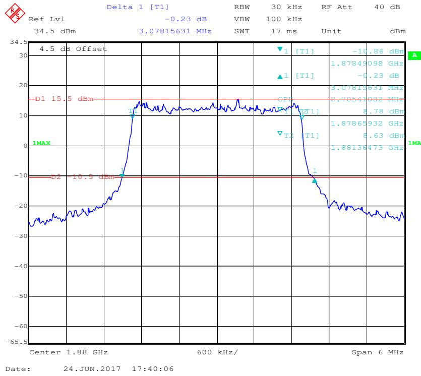
**16-QAM (3.0 MHz) - 99% Occupied Bandwidth &26 dB Bandwidth, Middle channel**
