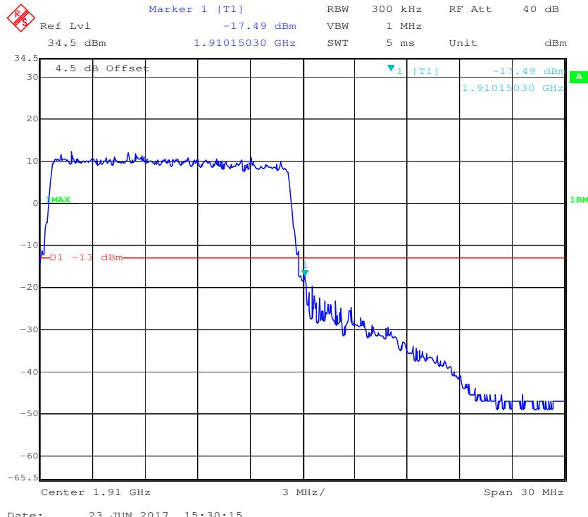
**16-QAM (15.0 MHz, FULL RB) - Left Band Edge**
