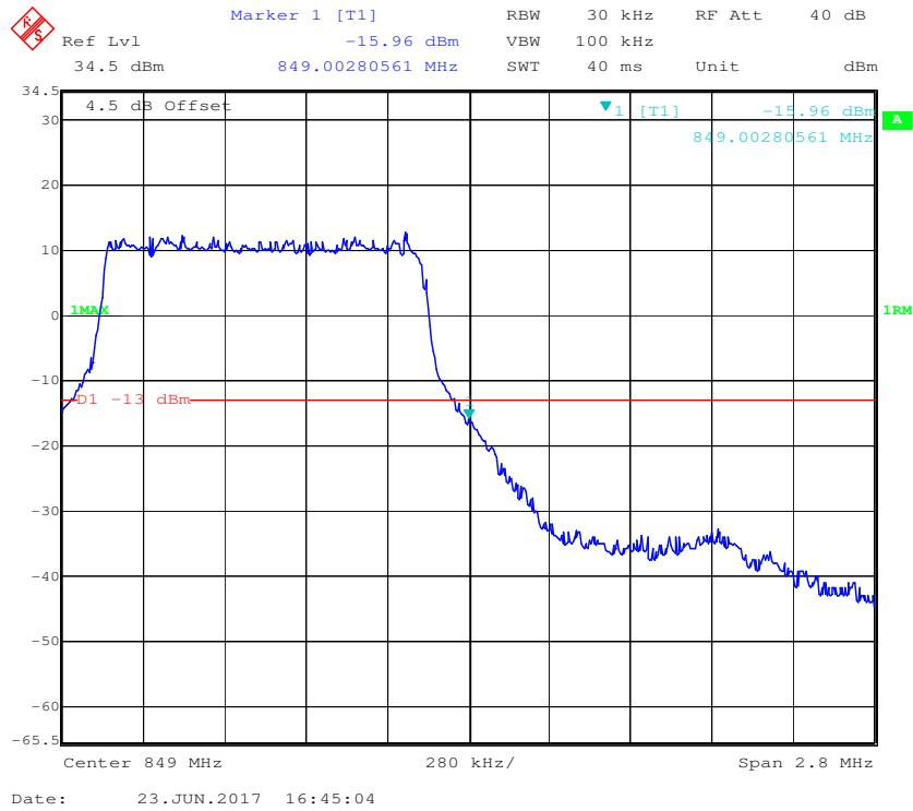
**16-QAM (1.4 MHz, FULL RB) - Left Band Edge**
