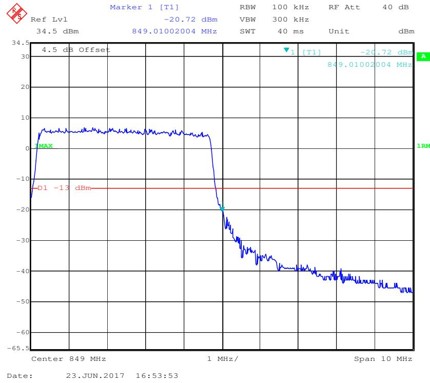
**QPSK (10.0 MHz, FULL RB) - Left Band Edge**
