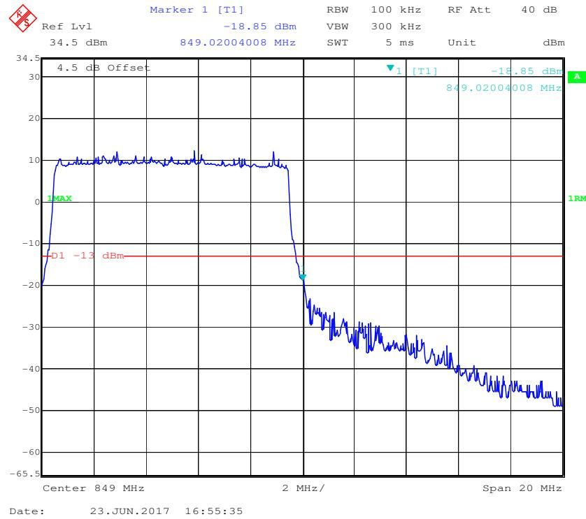
**16-QAM (10.0 MHz, FULL RB) - Left Band Edge**
