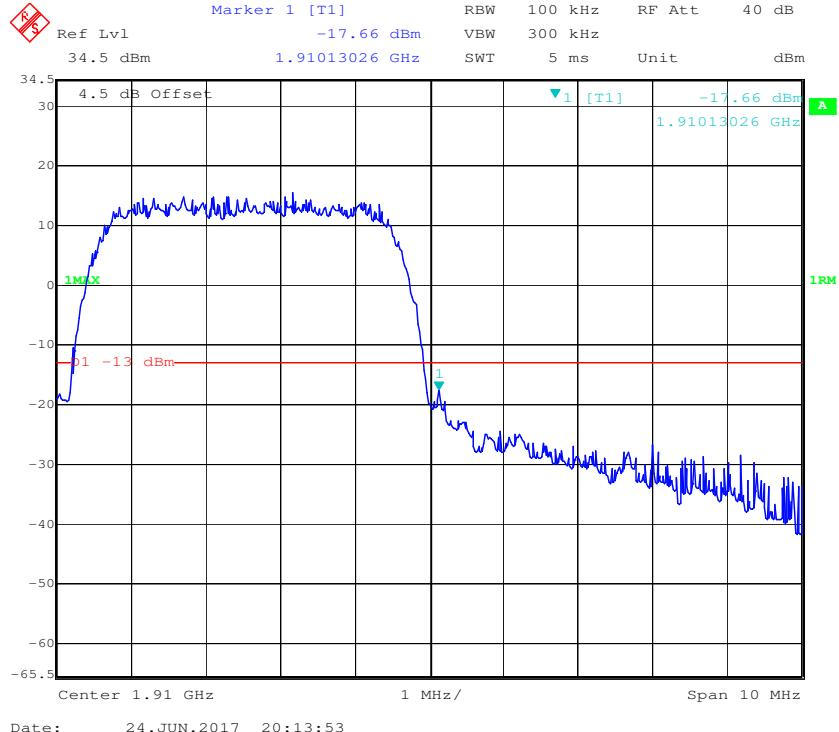
**PCS Band, Left Band Edge for HSUPA (BPSK) Mode**
