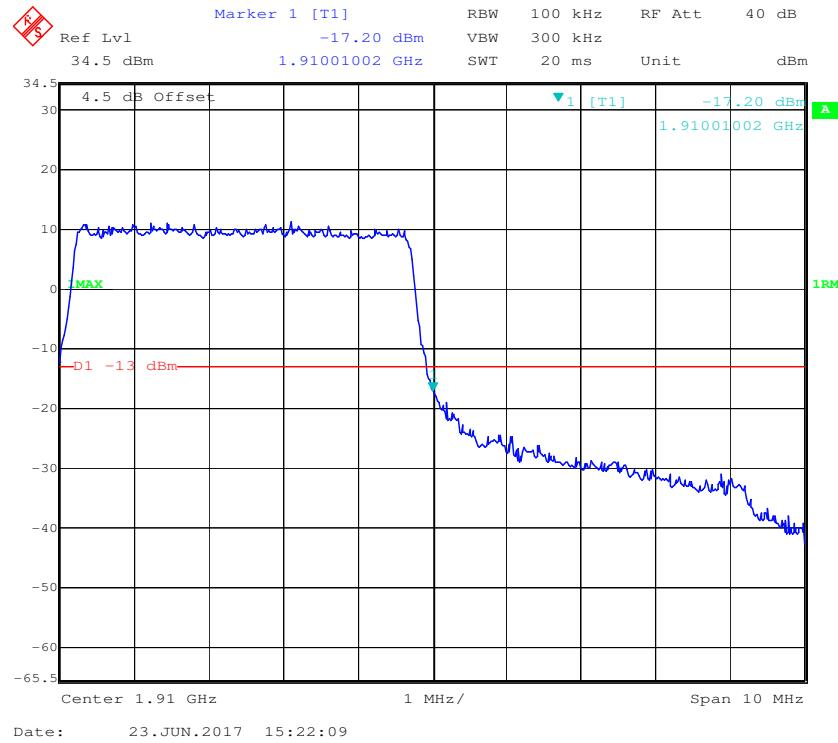
**16-QAM (5.0 MHz, FULL RB) - Left Band Edge**
