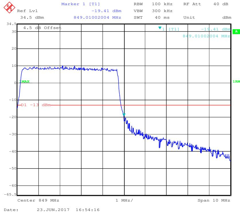
**16-QAM (5.0 MHz, FULL RB) - Left Band Edge**
