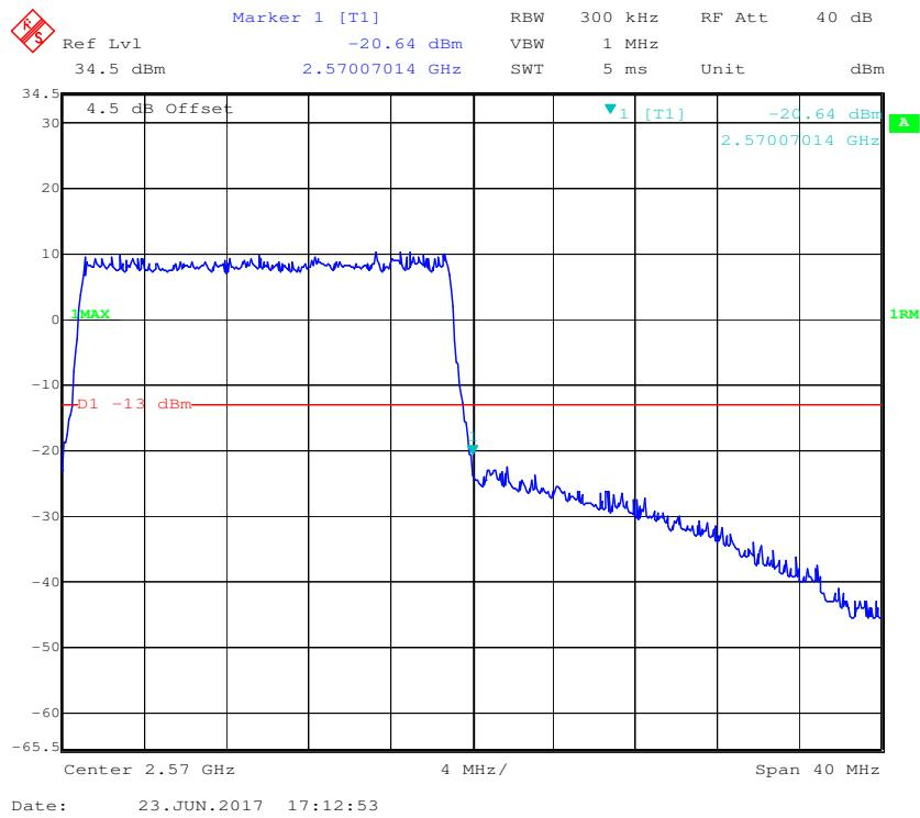
**16-QAM (20 MHz, FULL RB) - Left Band Edge**
