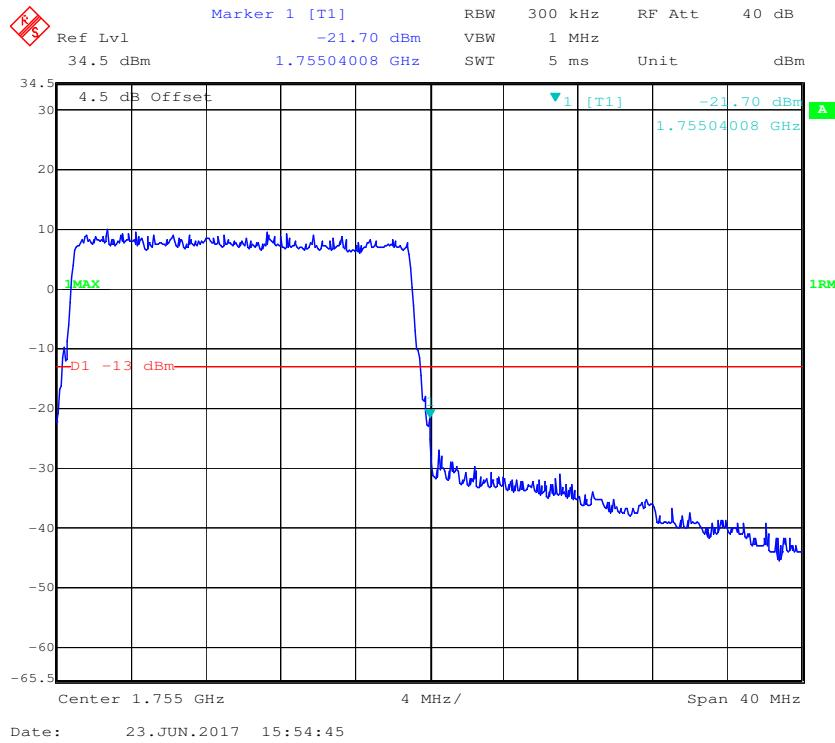
**LTE Band 5:****QPSK (1.4 MHz, FULL RB) - Left Band Edge**
