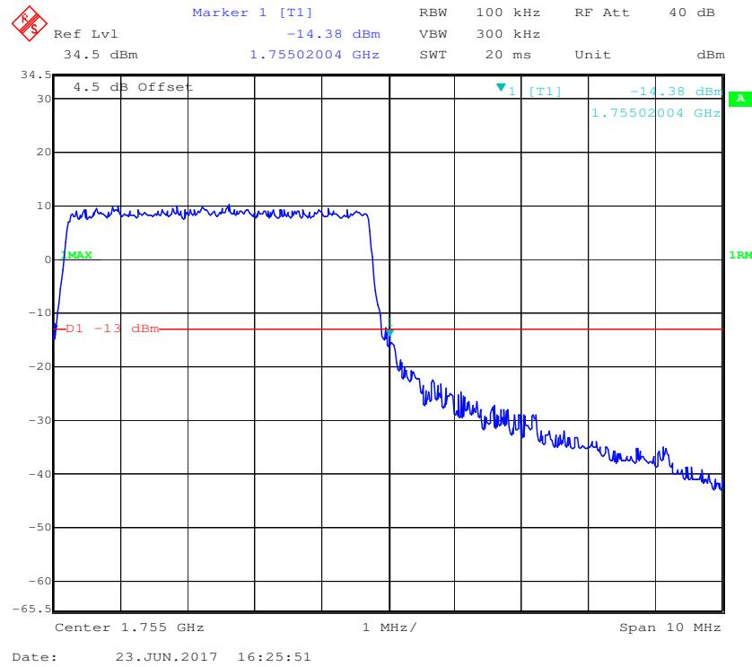
**QPSK (10.0 MHz, FULL RB) - Left Band Edge**
