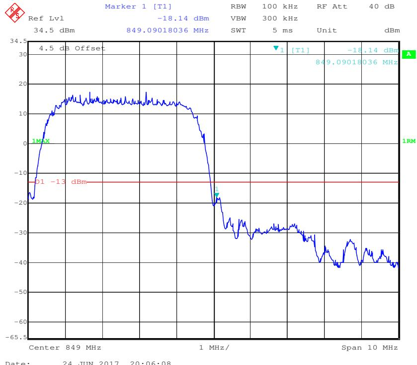
**Cellular Band, Left Band Edge for HSDPA (16QAM) Mode**
