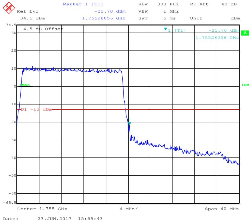
**16-QAM (20.0 MHz, FULL RB) - Left Band Edge**
