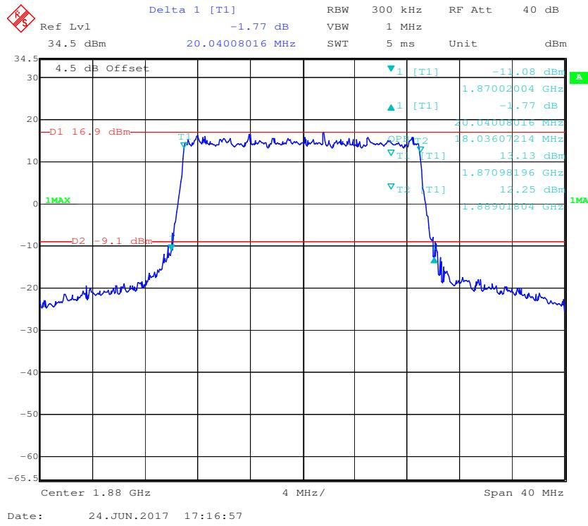
**16-QAM (20.0 MHz) - 99% Occupied Bandwidth & 26 dB Bandwidth, Middle channel**
