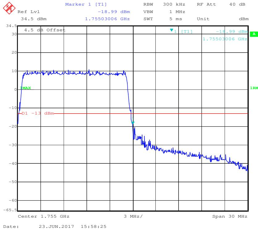
**QPSK (20.0 MHz, FULL RB) - Left Band Edge**
