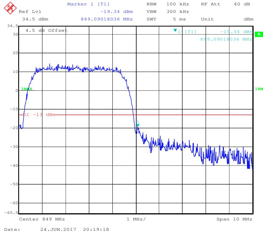
**PCS Band, Left Band Edge for GSM (GMSK) Mode**
