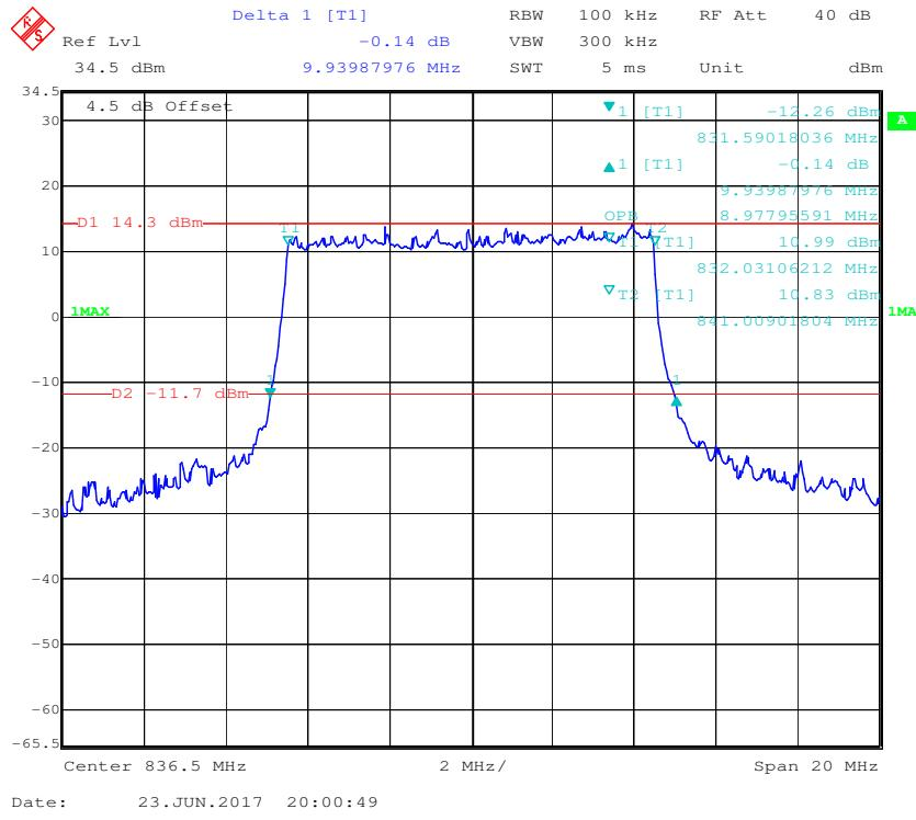
**16-QAM (10.0 MHz) - 99% Occupied Bandwidth & 26 dB Bandwidth, Middle channel**
