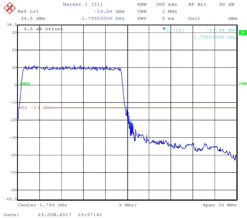
**16-QAM (15.0 MHz, FULL RB) - Left Band Edge**
