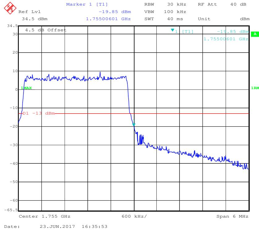
**QPSK (5.0 MHz, FULL RB) - Left Band Edge**
