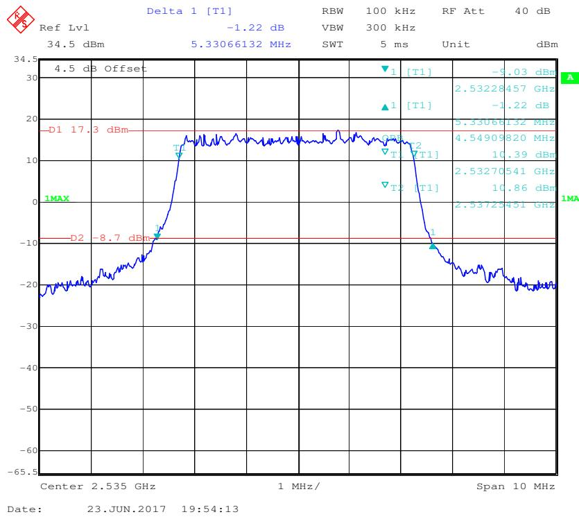
**16-QAM (5 MHz) - 99% Occupied Bandwidth &26 dB Bandwidth, Middle channel**
