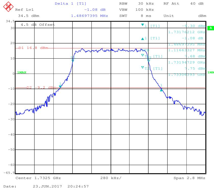
**16-QAM (1.4 MHz) - 99% Occupied Bandwidth &26 dB Bandwidth, Middle channel**
