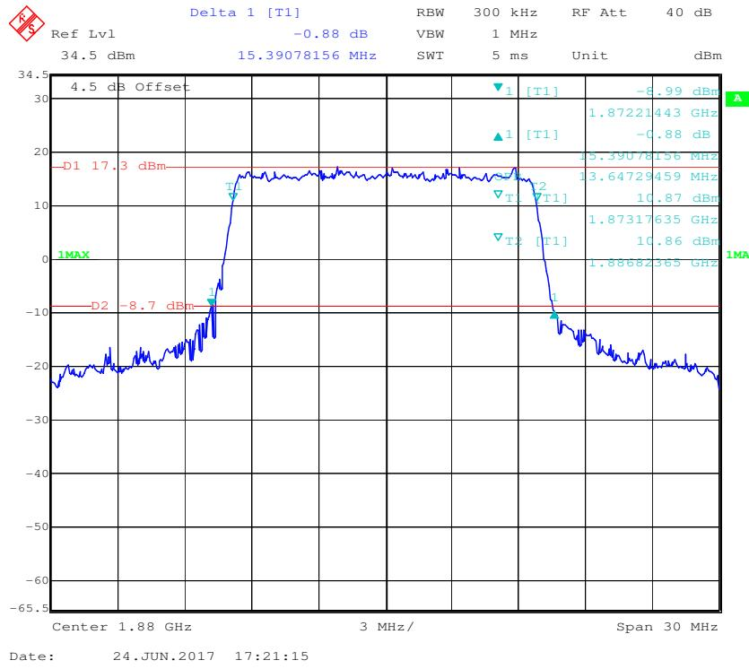
**16-QAM (15.0 MHz) - 99% Occupied Bandwidth &26 dB Bandwidth, Middle channel**
