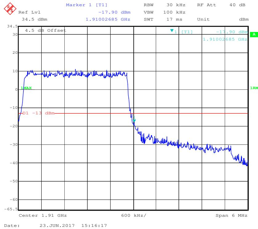
**16-QAM (3.0 MHz, FULL RB) - Left Band Edge**
