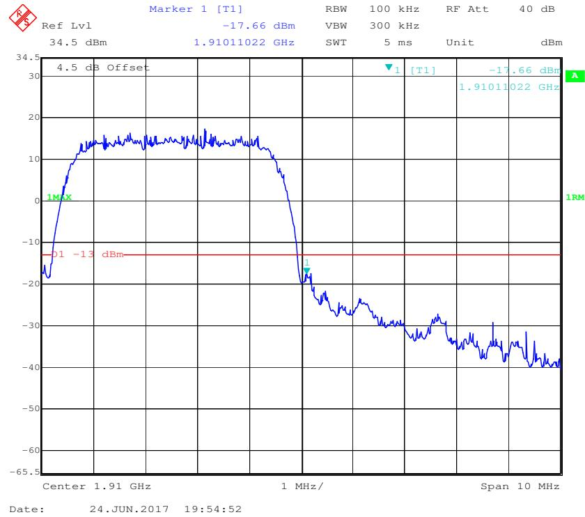
**PCS Band, Left Band Edge for HSDPA (16QAM) Mode**
