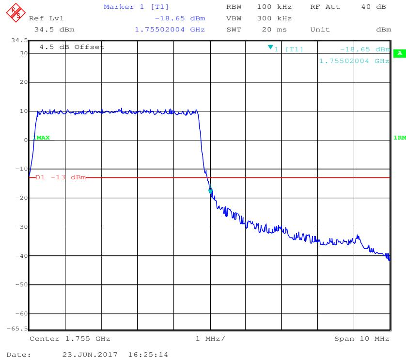
**16-QAM (5.0 MHz, FULL RB) - Left Band Edge**
