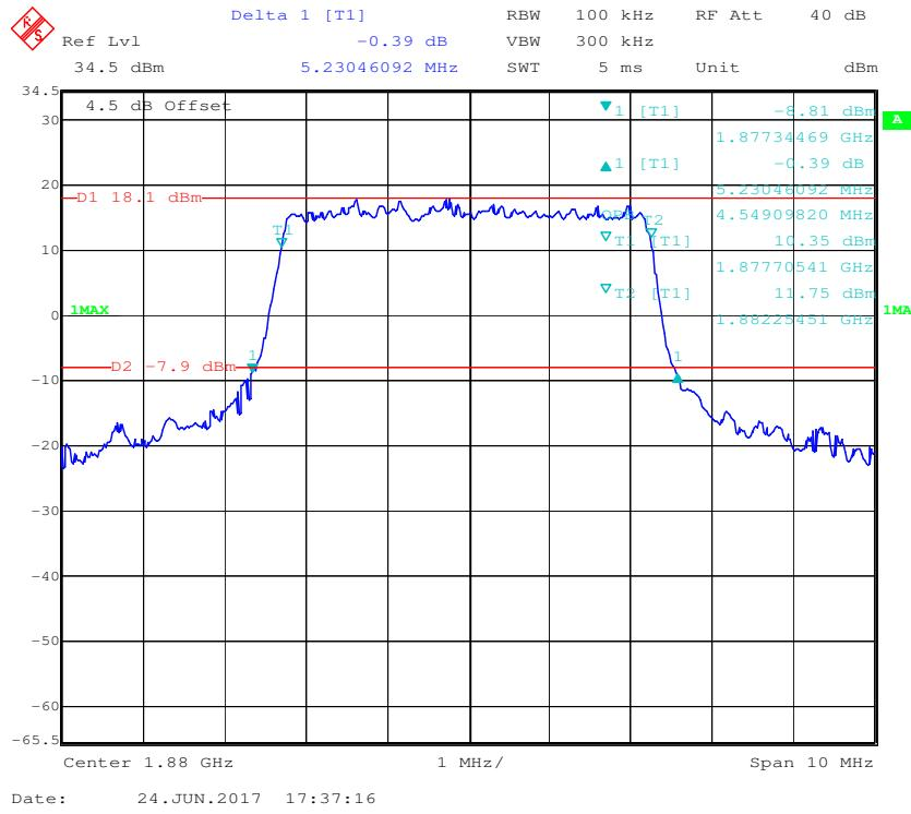
**16-QAM (5.0 MHz) - 99% Occupied Bandwidth &26 dB Bandwidth, Middle channel**
