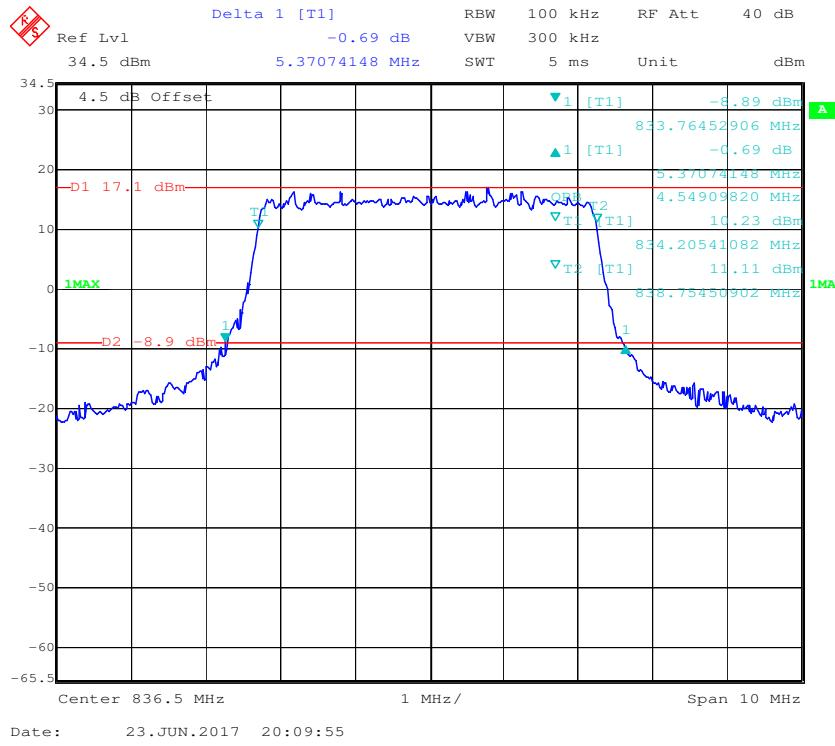
**16-QAM (5.0 MHz) - 99% Occupied Bandwidth &26 dB Bandwidth, Middle channel**
