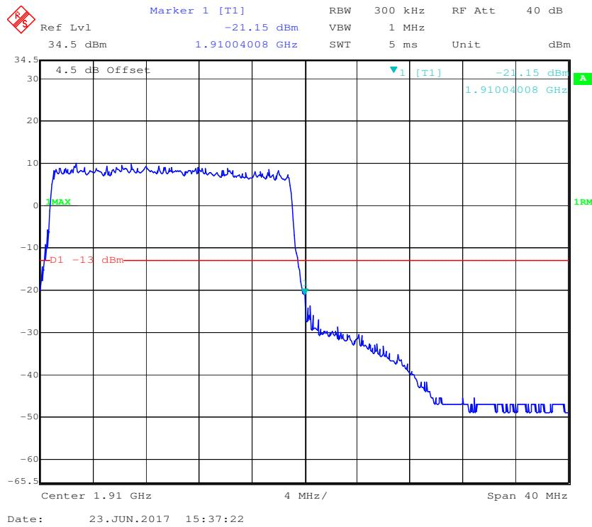
**LTE Band 4:****QPSK (1.4 MHz, FULL RB) - Left Band Edge**
