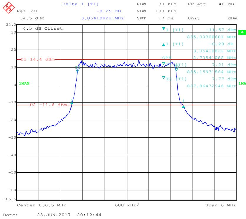
**16-QAM (3.0 MHz) - 99% Occupied Bandwidth &26 dB Bandwidth, Middle channel**
