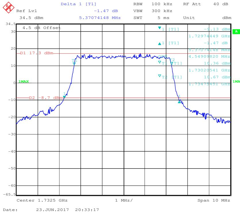
**16-QAM (5.0 MHz) - 99% Occupied Bandwidth &26 dB Bandwidth, Middle channel**
