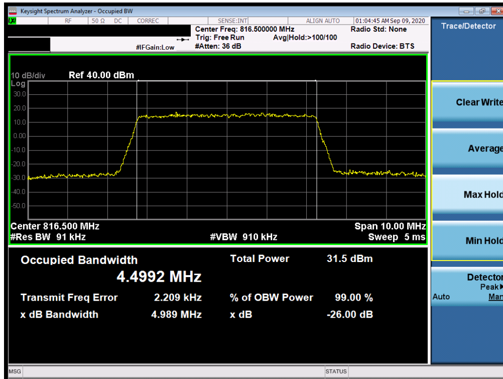
Plot 7-7. Occupied Bandwidth Plot (LTE Band 26 - 5MHz QPSK - Full RB Configuration)
