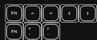
FN + ↑/↓ Backlight brightness + - FN + → Backlight color switching
