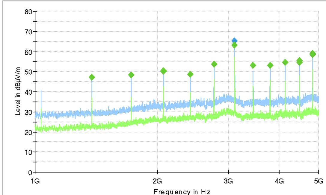
**Plot 4: Radiated Emissions (1GHz-5GHz) scanned at 3m SAC**
