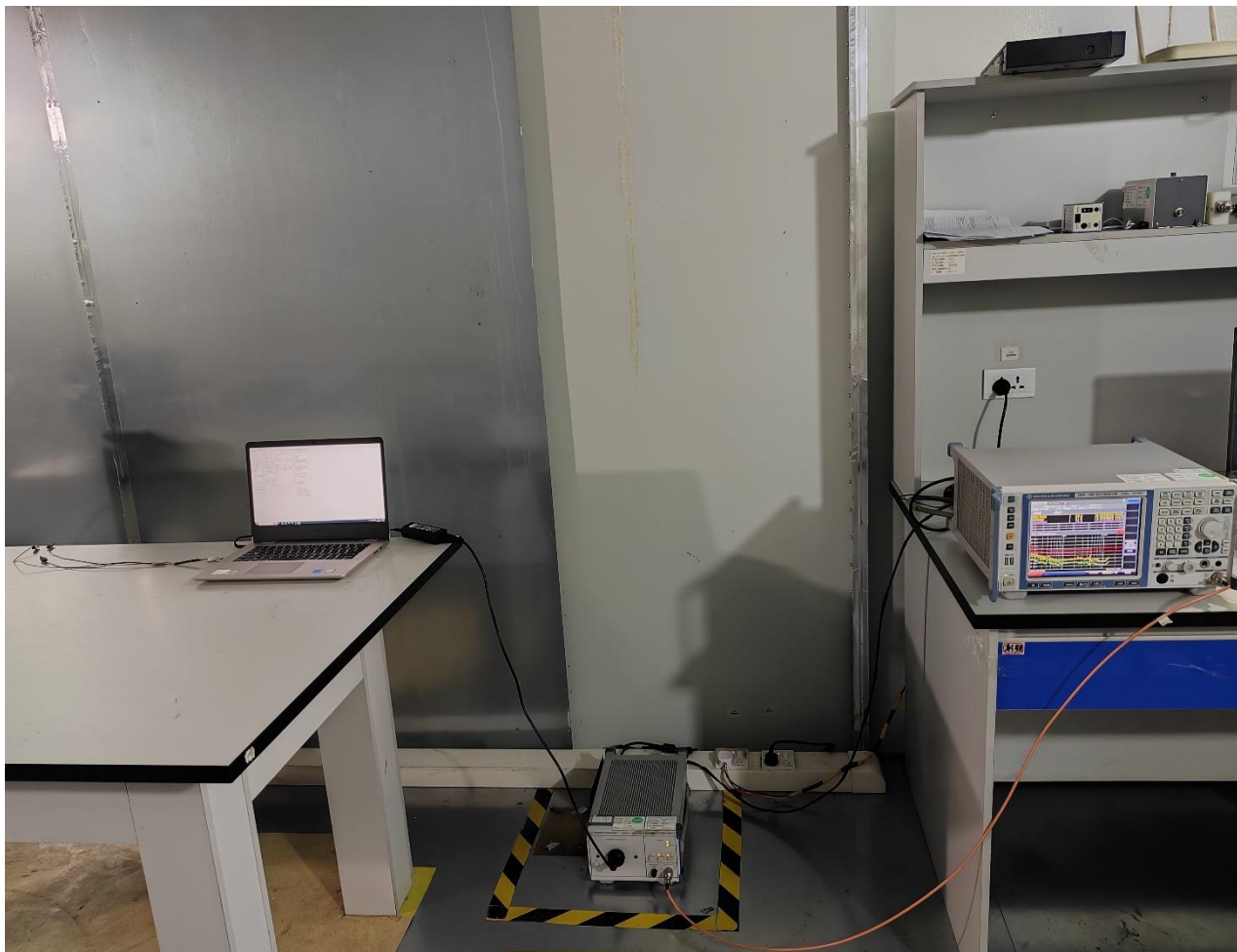
Photograph 3: Set-up for Conducted Emission on AC Mains
