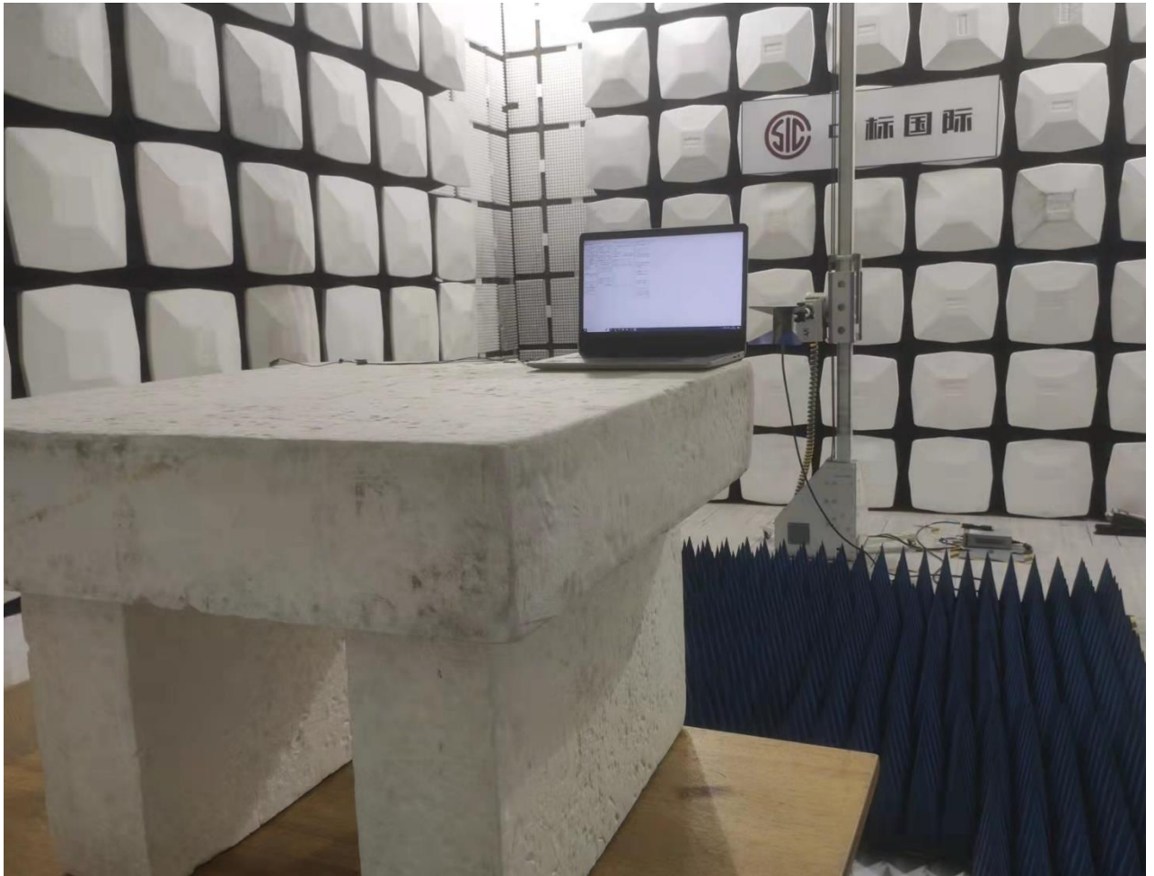
Photograph 2: Set-up for Radiated Spurious Emission, Above 1GHz
