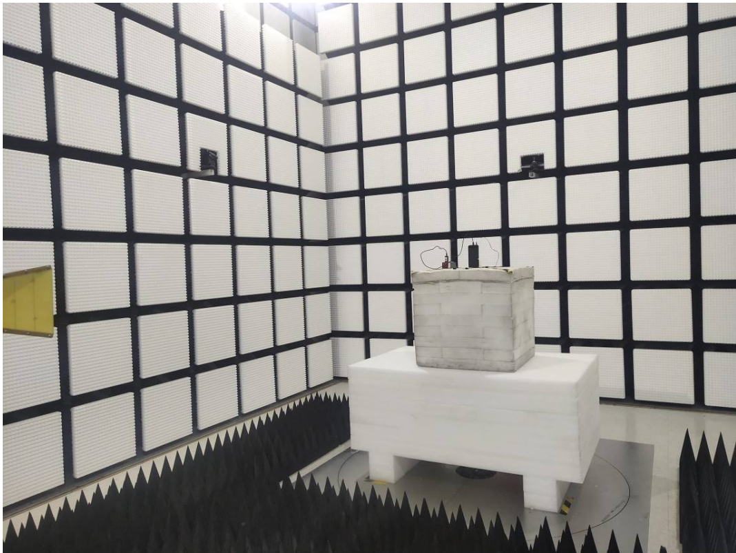
Radiated Emission Above 1GHz View Adapter 1#
