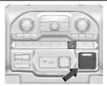
In Cab Power Outlet and DC/AC Switch
