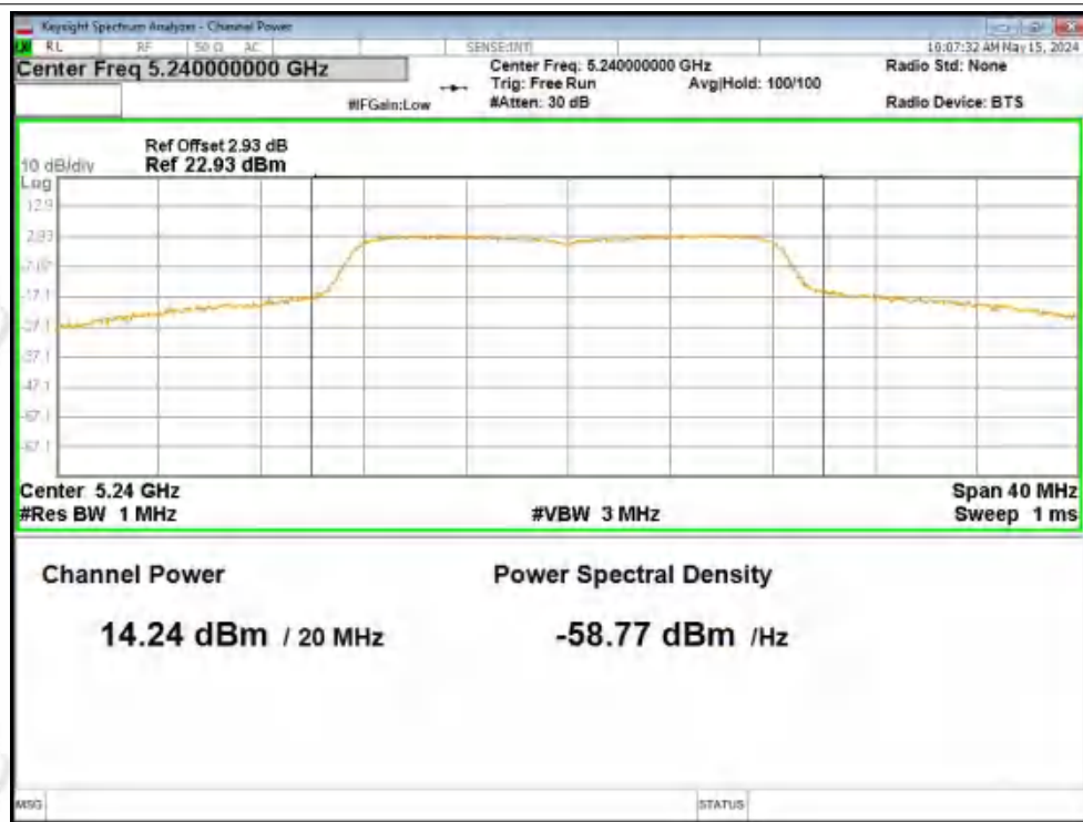
Power NVNT a 5240MHz Ant2
