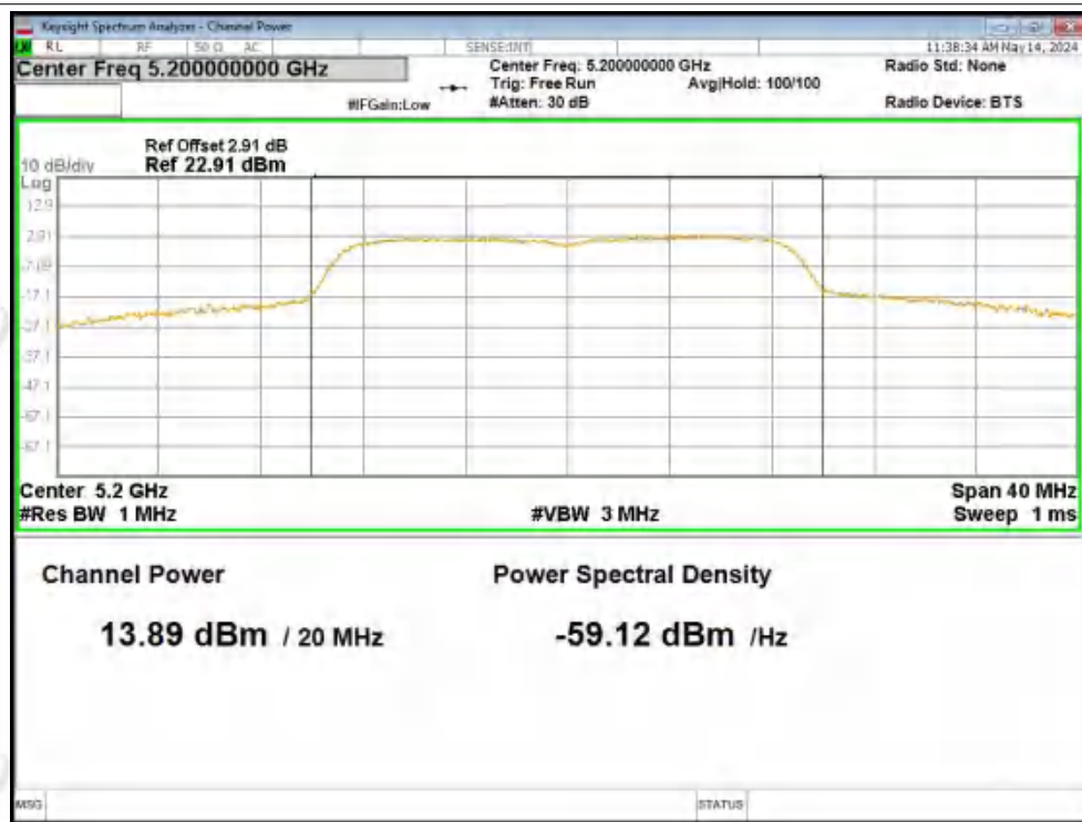
Power NVNT n20 5200MHz Ant1
