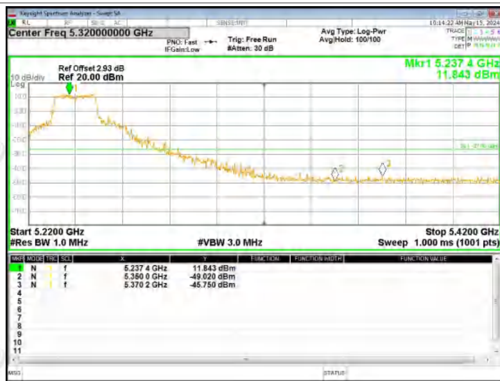
Band Edge NVNT n20 5240MHz High Ant2
