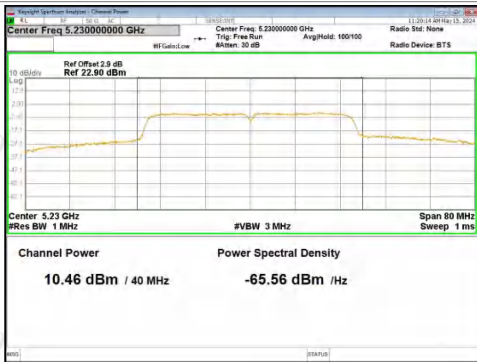
Power NVNT ac40 5230MHz Ant1
