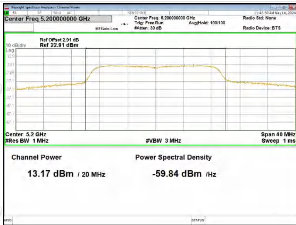
Power NVNT ac20 5200MHz Ant1
