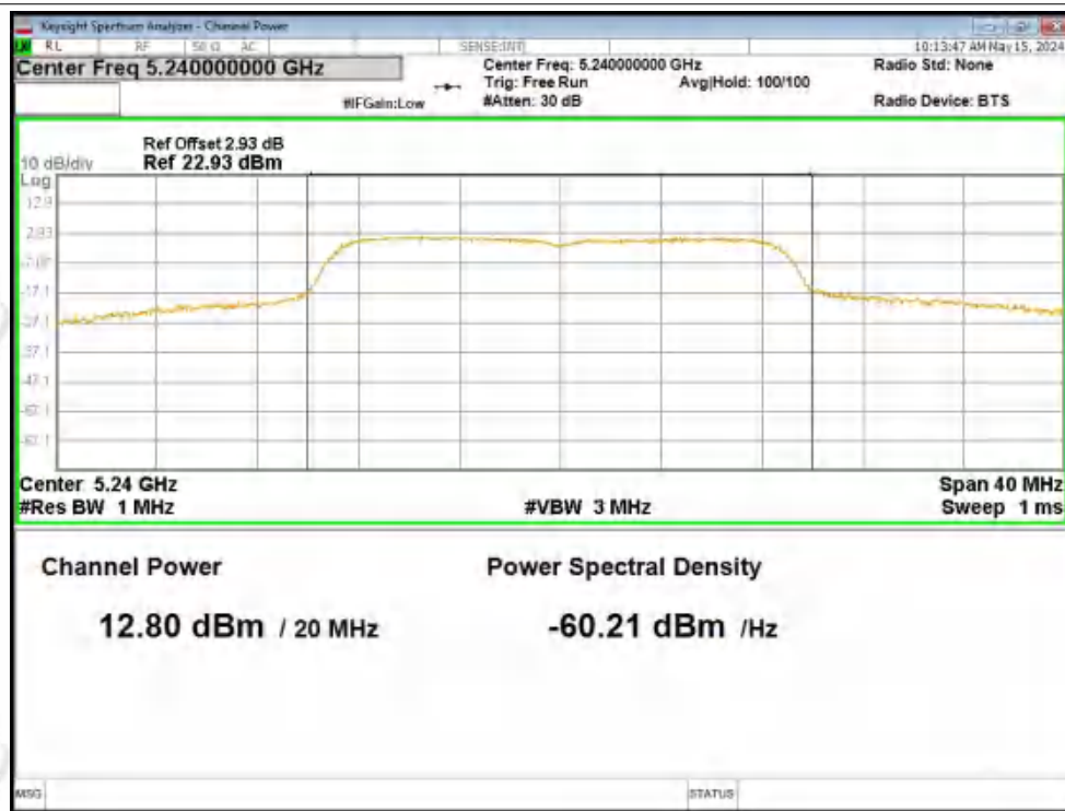
Power NVNT n20 5240MHz Ant2
