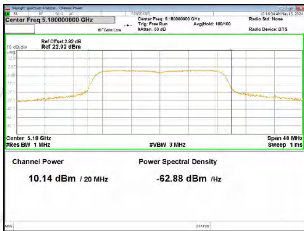
Power NVNT ac20 5180MHz Ant2
