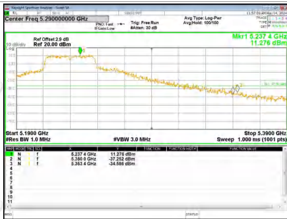
Band Edge NVNT n40 5230MHz High Ant1
