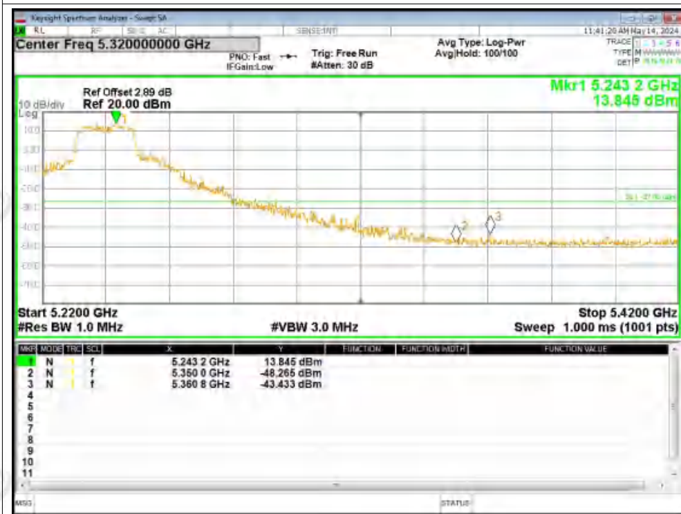
Band Edge NVNT n20 5240MHz High Ant1
