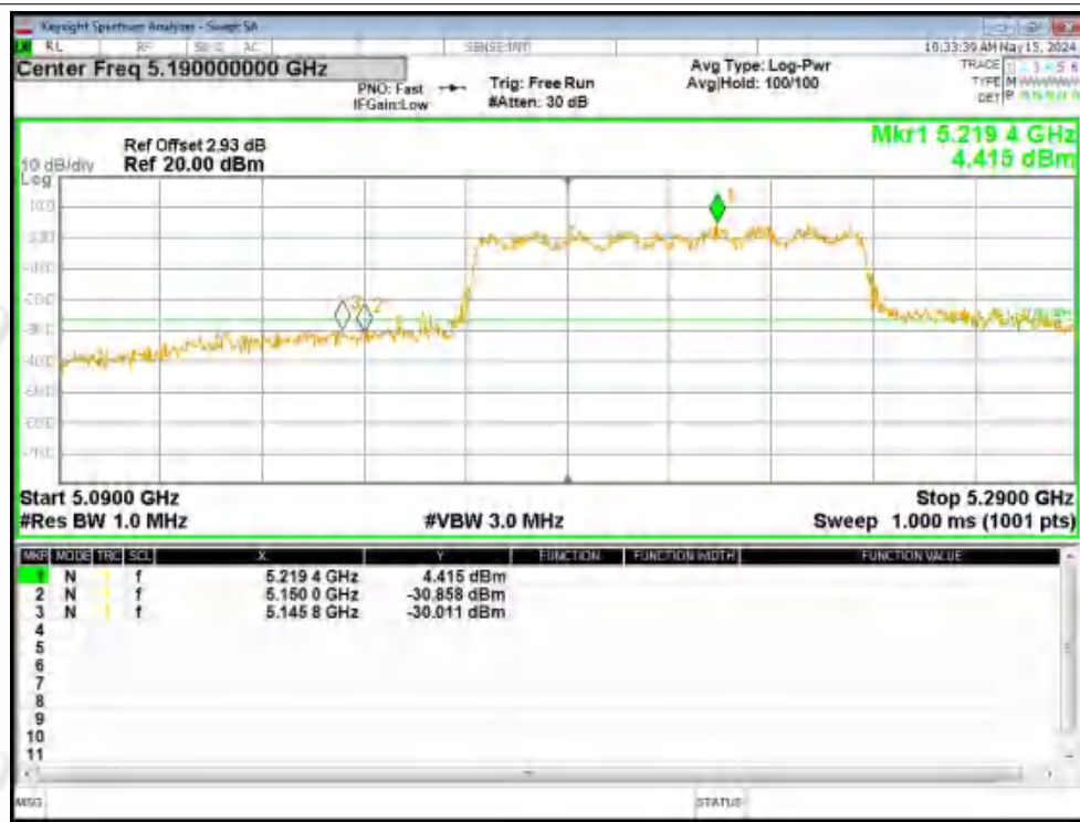
Band Edge NVNT ac80 5210MHz Low Ant2
