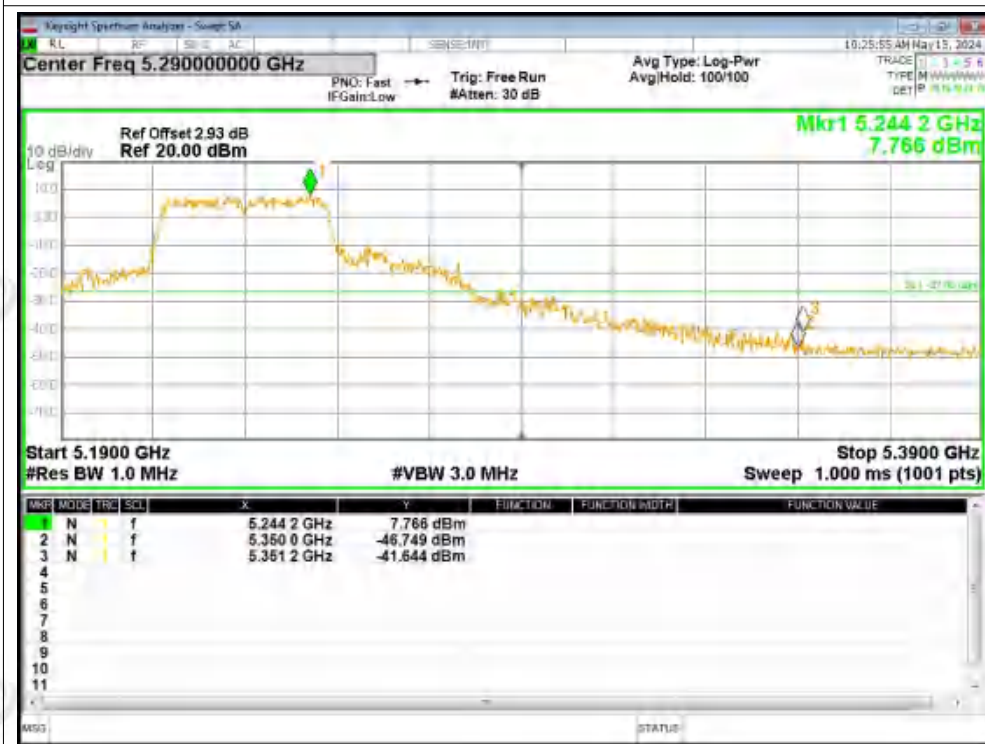
Band Edge NVNT n40 5230MHz High Ant2
