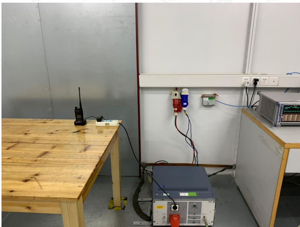
RADIATED EMISSION TEST SETUP-BELOW 1GHZ
