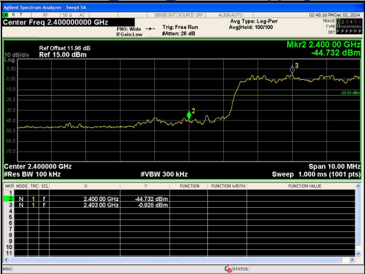
Out Of Band Emission(Left) 8DPSK_3-DH5_Channel Hopping
