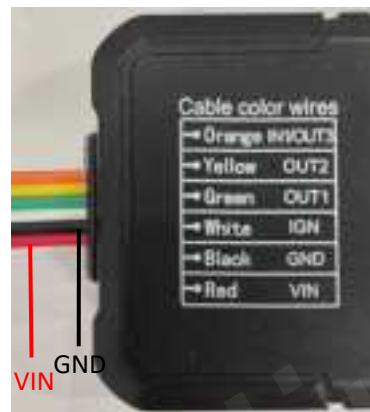
Figure 3: Typical Power Connection
