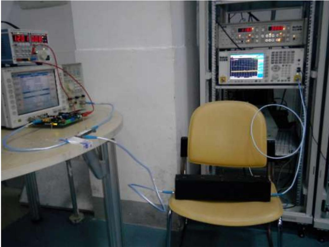
Frequency Stability Under Temperature & Voltage Variations Setup
