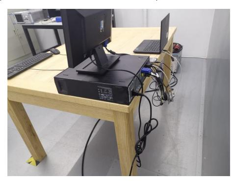
Test Mode: Mode 2 Description: Front view of Radiated Emission Test Setup
