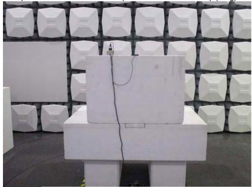
Description: Back View of Radiated Spurious Emission Test Setup (Bilog)
