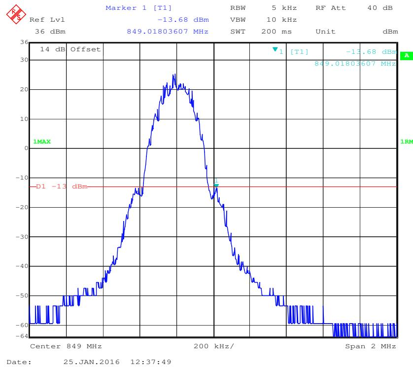
**PCS Band, Left Band Edge for GSM (GMSK) Mode**
