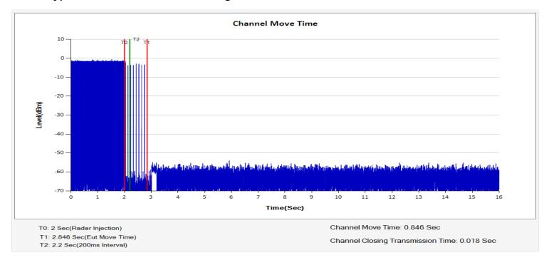
**Verdict:** Note: narrowing the sweep time as the good engineering process for the verification of transmission closing in 200ms
