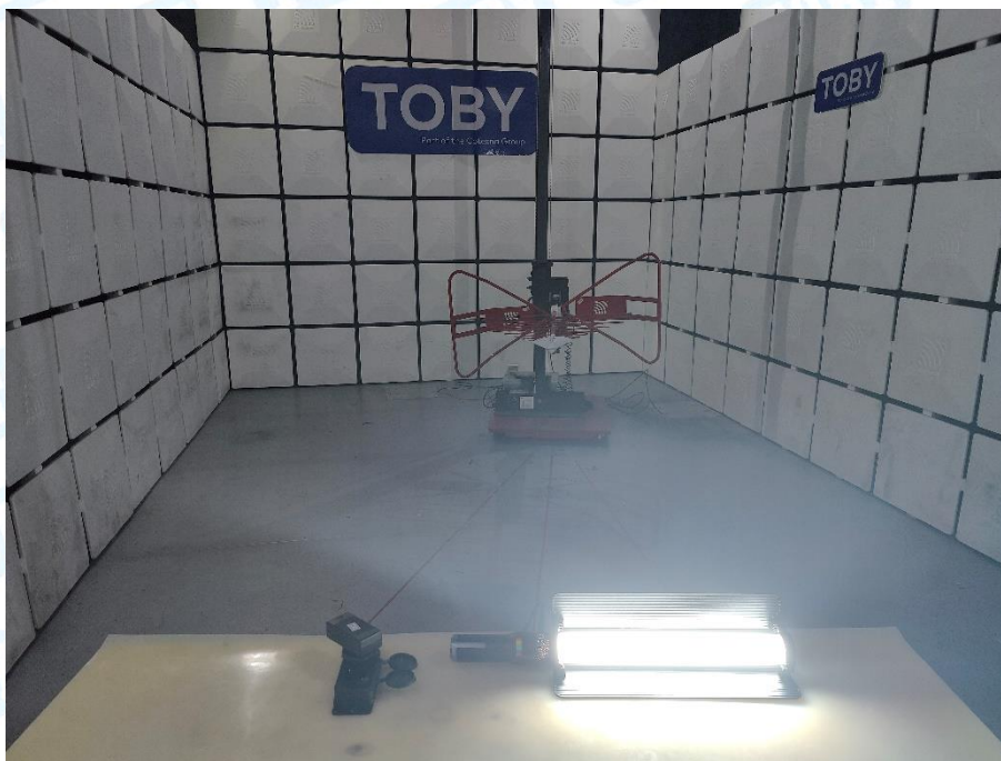
Photo of Setup for Radiated Emission (30MHz~1GHz)
