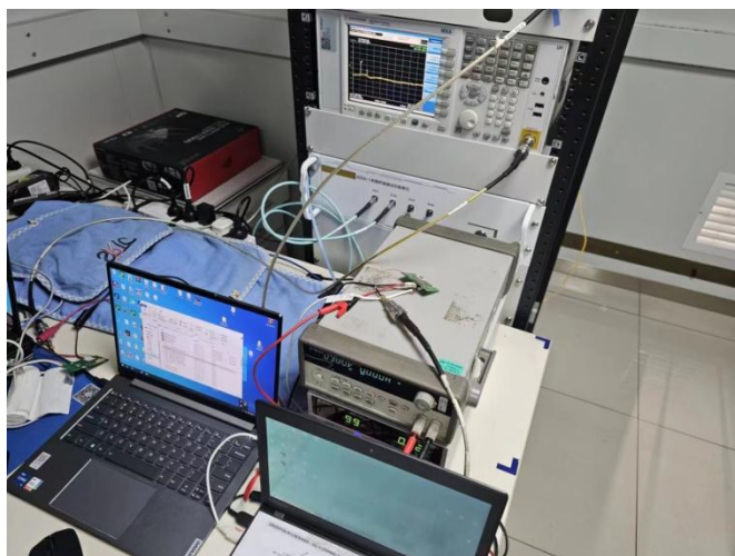
RF Conducted Test setup (BT/WIFI)
