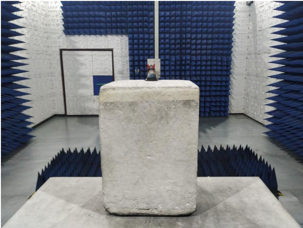
RADIATED EMISSION TEST SETUP ABOVE 1GHZ
