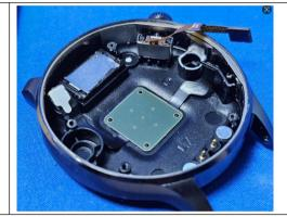
The antenna is Metal mid-frame antenna.
