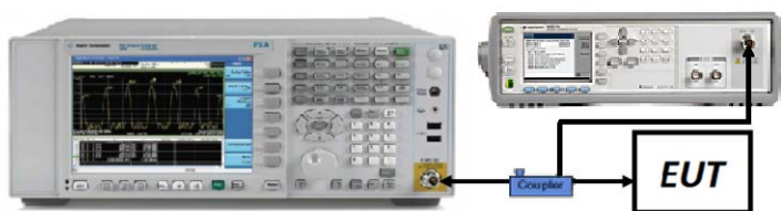
Figure 7-5. Test Instrument & Measurement Setup
