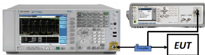
Figure 7-7. Test Instrument & Measurement Setup
