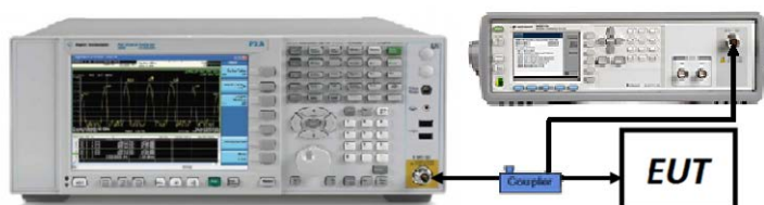
Figure 7-4. Test Instrument & Measurement Setup
