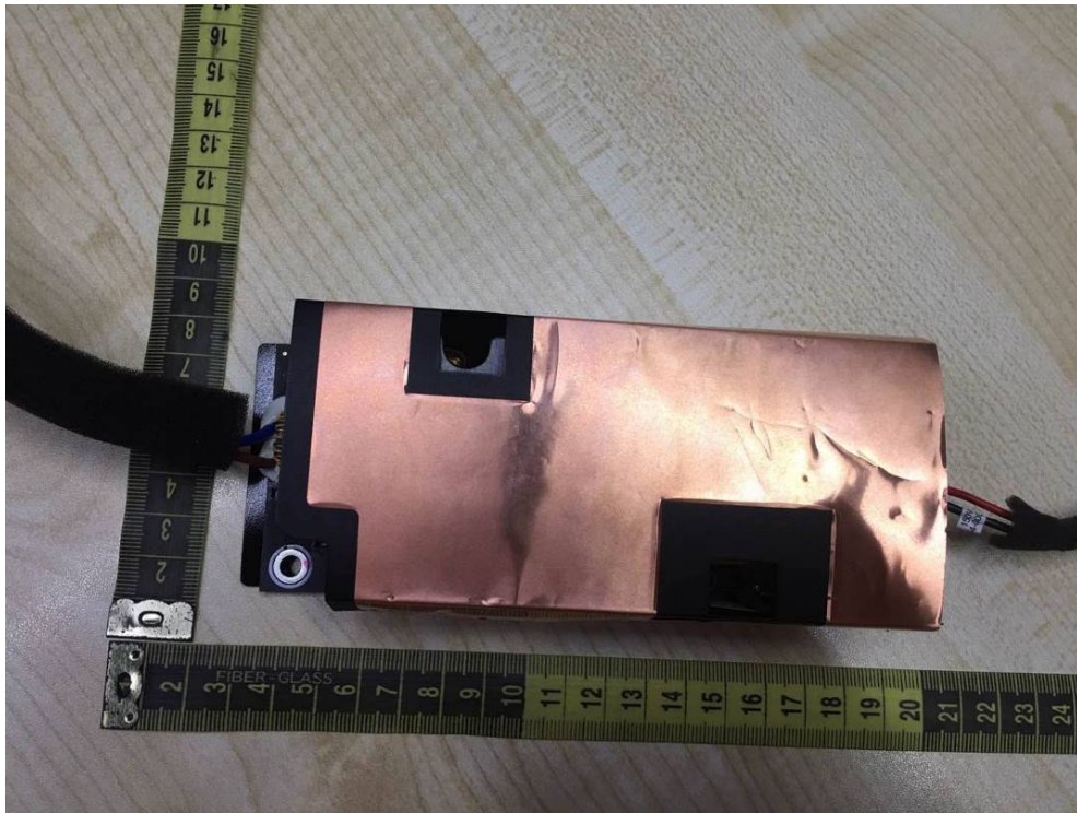
Fig. 7: Power board bottom view with Mylar sheet (in both active speaker and passive speaker)
