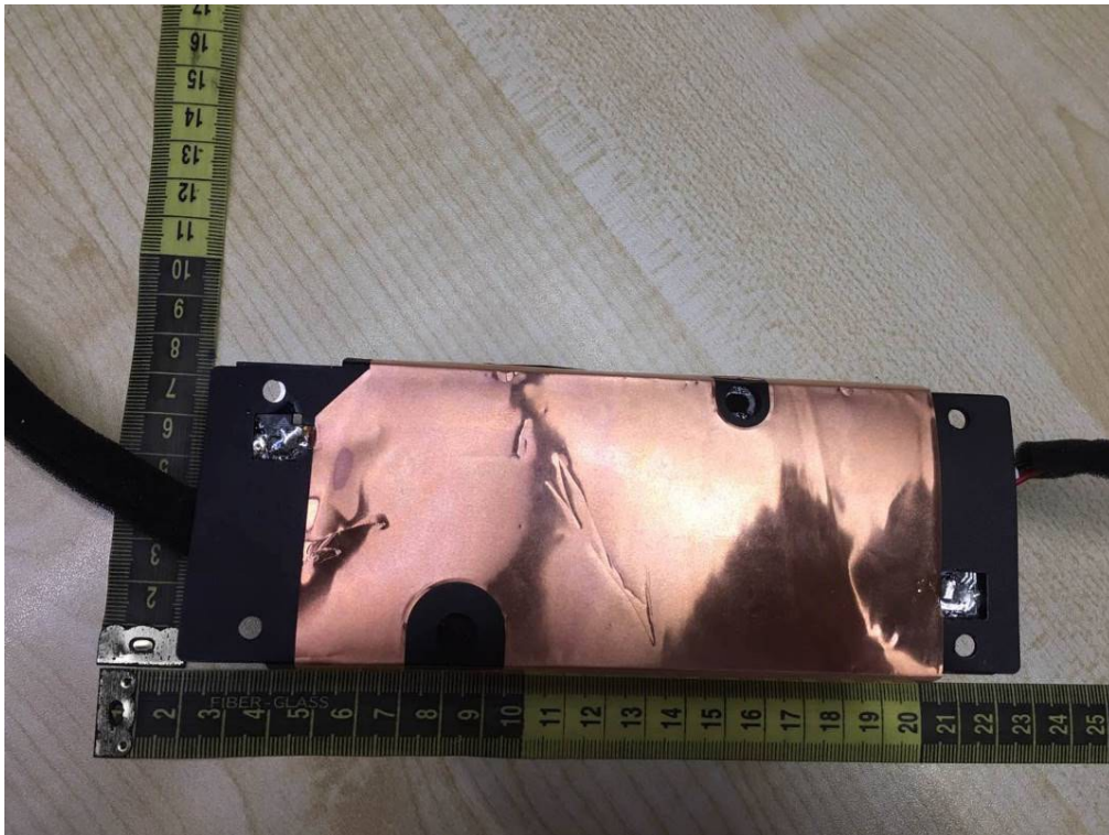
Fig. 6: power board top view with Mylar sheet (in both active speaker and passive speaker)
