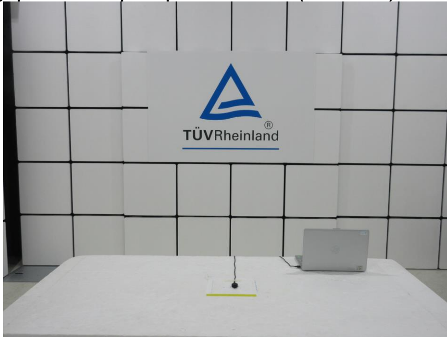
Photograph 2: Test Setup for Spurious Emissions (Front View 2)
