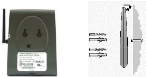
Figure 2-3 Mounting the Access Point on a wall
