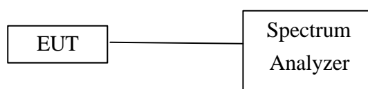
Figure 5: Output power and measurement configuration.
